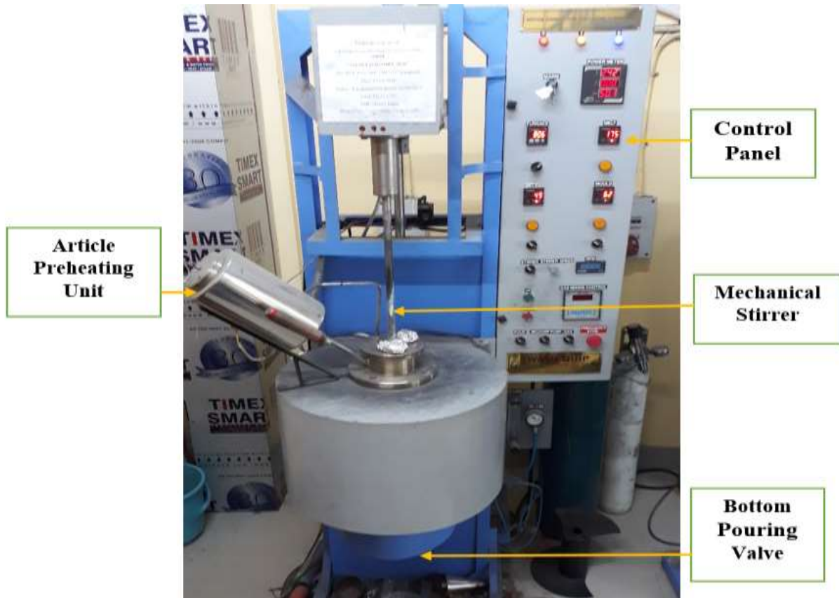
Figure 3.1. Bottom Poured Stir Casting Resistance Furnace [Courtesy Smart Foundry Lab: JU]
