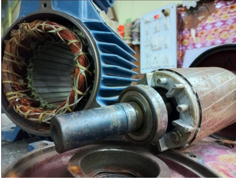
Fig. 7.1. Induction motor under experiment, with rotor pulled out.
