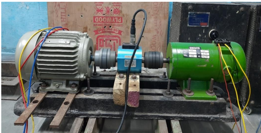
Fig. 6.4. Induction motor under experiment, coupled with DC generator through a torque transducer.
