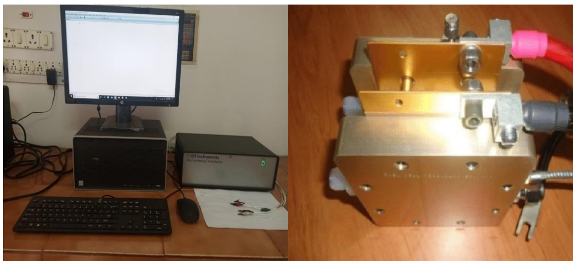
Figure 4.9: Single cell membrane electrode assembly setup with EIS work station.
