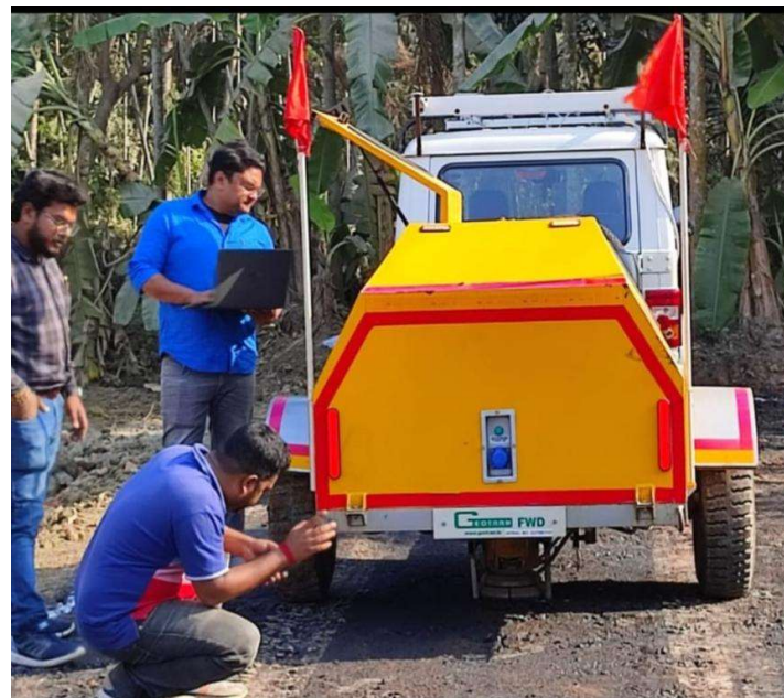
Fig. 6.26: FWD deflection recording on scrap tyre modified subgrade pavement
