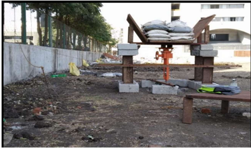
Fig. 2.3: Field CBR setup (After Dhorajiya et al 2019)
