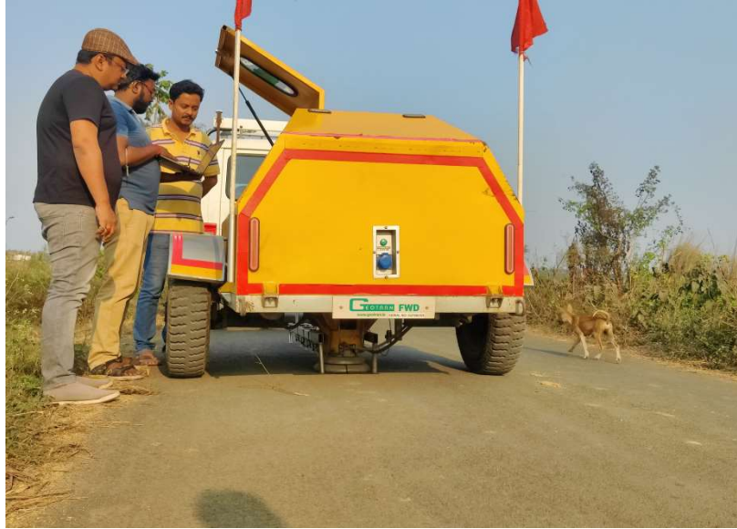
Fig. 6.25: FWD deflection recording on Jibantala -Taldi Road
