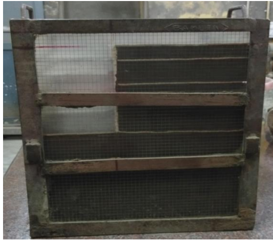
Figure 4.8 - Photographs of ground deformations before test and after rotation for 150 sec for case 14 (Excavation depth 14 m and 3 struts)
