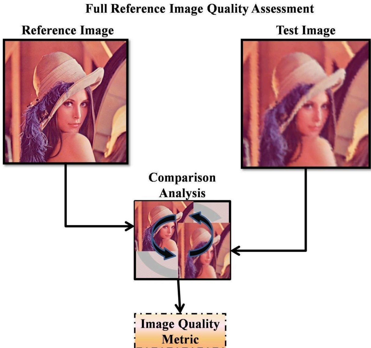
Figure 2.2: Overview of the process of Full-reference Image Quality Assessment
