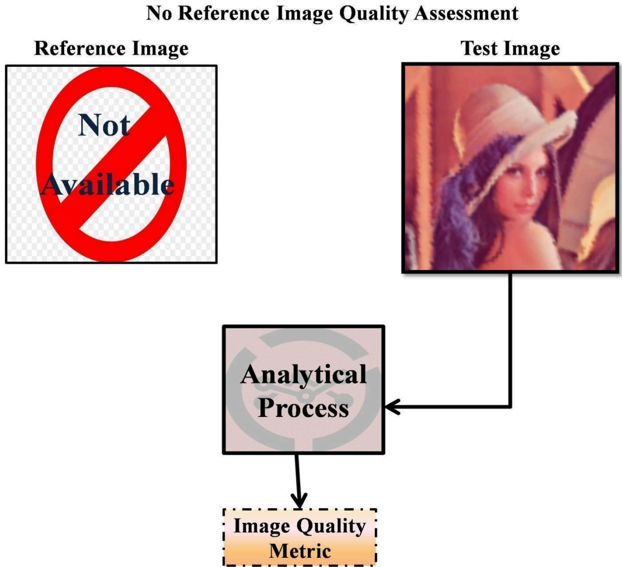
Figure 2.4: Overview of the process of No-Reference Image Quality Assessment (NRIQA)
