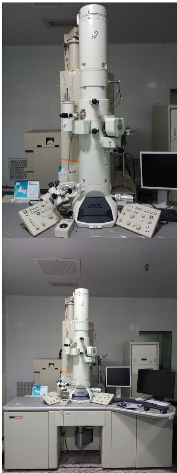
Fig 1.11: Transmission electron microscope instrument
