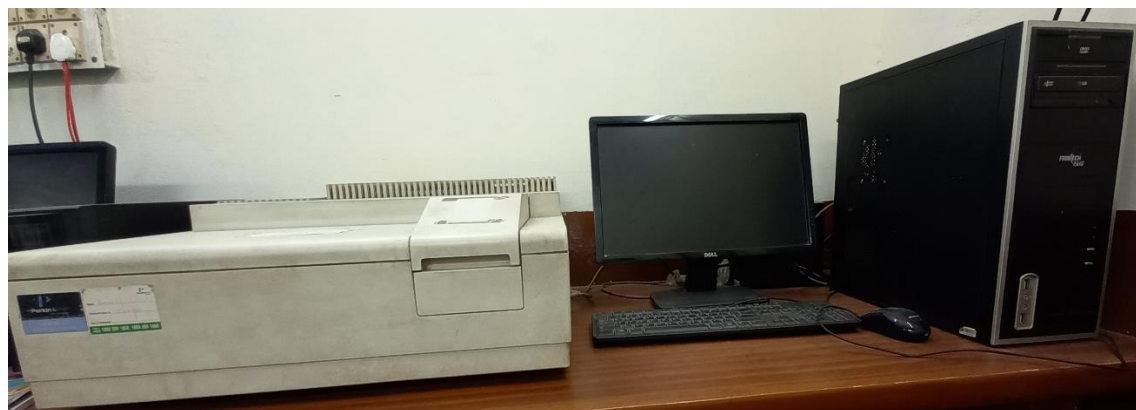
Fig 1.12: UV- Vis Spectrophotometer used for analysis of the sample
