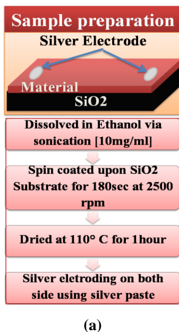
Figure 2.20 Schematic of sample preparation (a); Morphology of samples coated upon Substrate (b), Inter electrode morphology (c)
