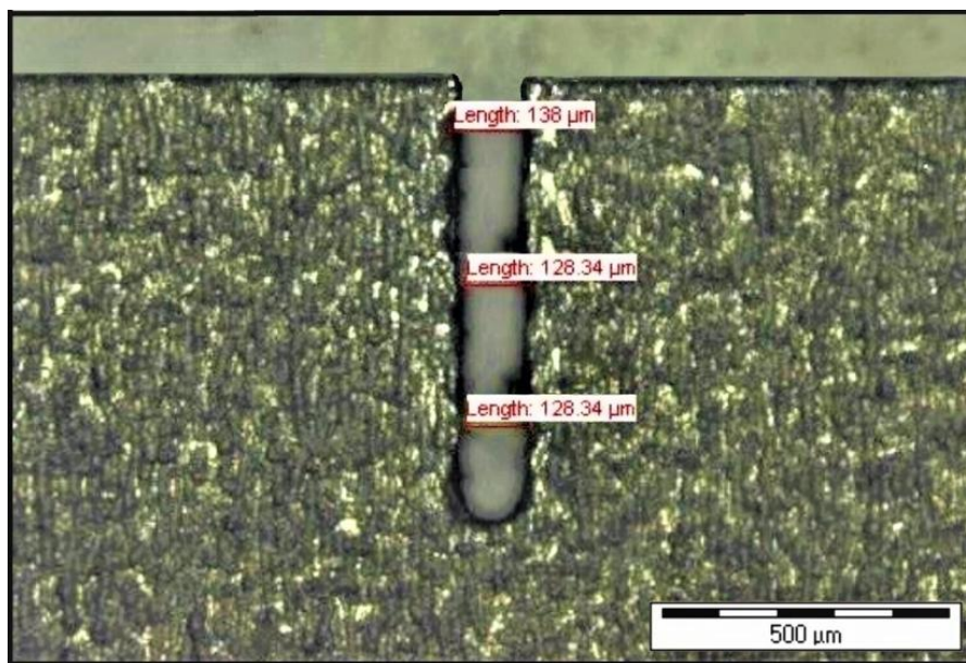
Figure 3.15 Machined nitinol SMA microslit
