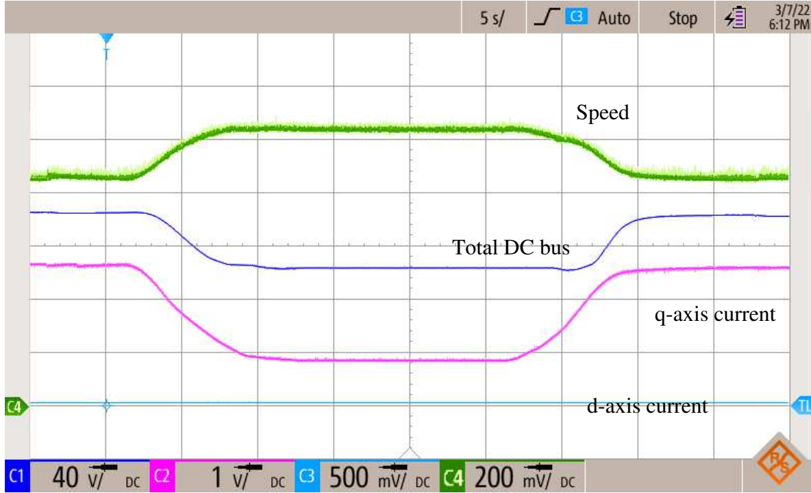
Fig 4.14: Speed control mode, speed variation from 900 rpm to 1050rpm and back: Ch. 1: Total DC bus voltage (40V/div); Ch. 2: q-axis current from DAC (1V/div); Ch. 3: d-axis current from DAC (0.5V/div); Ch. 4: Speed change from 900 rpm to 1050 rpm and back;
