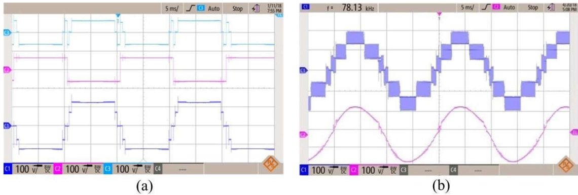
Fig. 3.9 Experimental waveforms: (a) top: voltage across terminals A & N; mid: voltage across terminals B & N; bot: voltage across terminals A & B; (b) top: voltage across terminals A & B'; bot: output voltage across load
