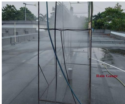
Fig. 3.4. Artificial Rain Simulation setup
