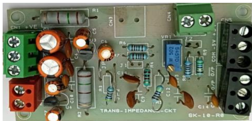
Fig. 3.16. Transimpedance with comparator circuit
