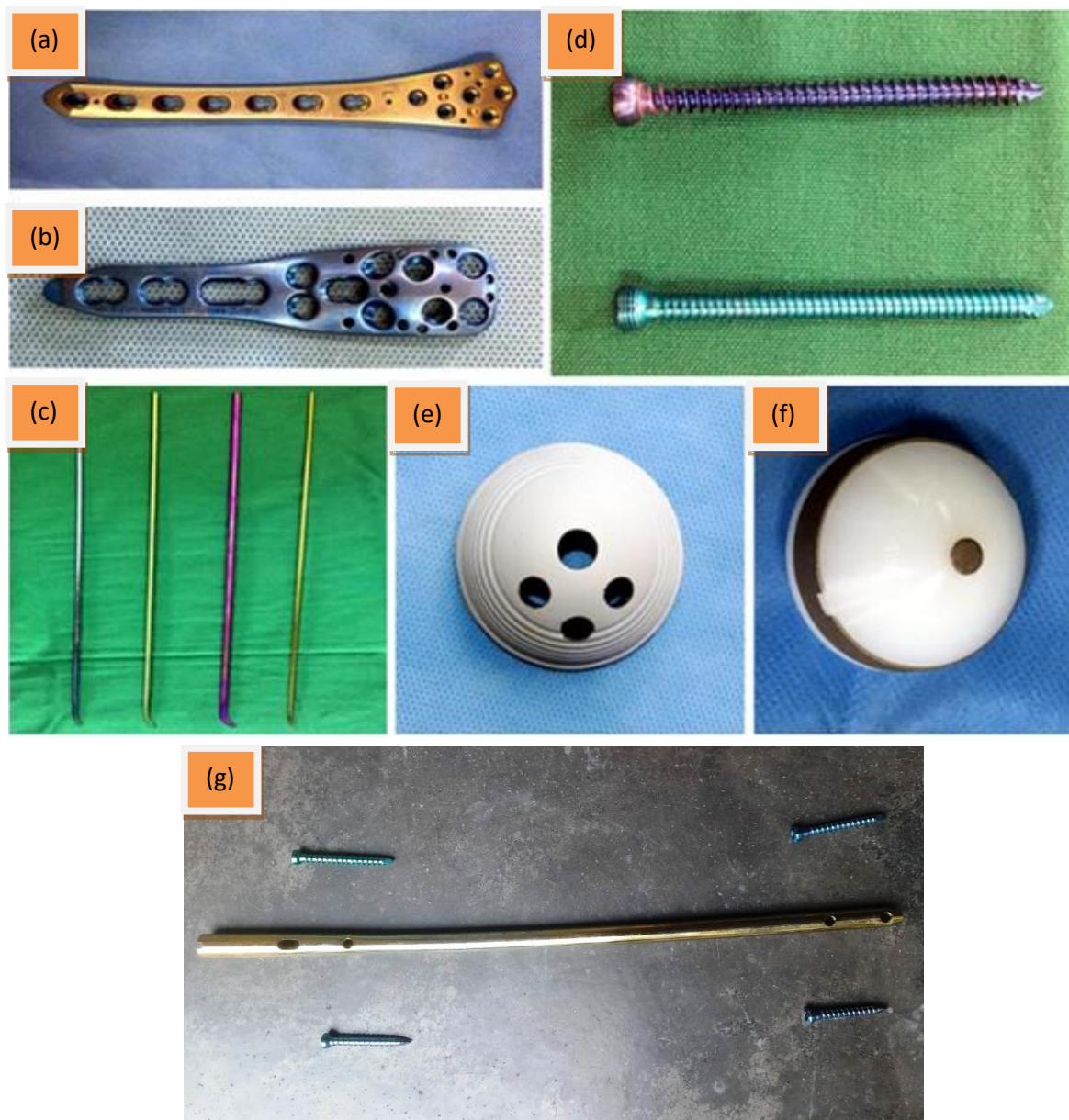
Fig.1.3: Uses of Titanium scaffolds for in orthopedics bone replacement and supports: (a) Compression plate for distal femoral locking; (b) Internal locking plate for proximal humerus fractures; (c) Titanium elastic nails for pediatric long bone fractures; (d) Locking and non-locking screws; (e) Titanium acetabular cup with HA coating for THR; (f) Polyethylene liner with a titanium lining on its rim (the polyethylene liner is fitted into the acetabular cup and represents as a acetabular component togetherly of THR ( Ghosh et al., 2018 ) & (g) screws and main rod for broken bone surgery (collected from Dishari Hospital, Malda).
