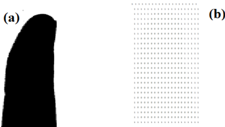
Fig.2.4.(a) Binary image of the finger. (b) Image matrix of the finger.
