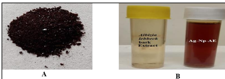
Fig. 2.1 Albizia lebbbeck stem bark extract powder (A); synthesized Silver nanoparticle with Pale-yellow and deep-brown solution of Ag-NP-AE (B).
