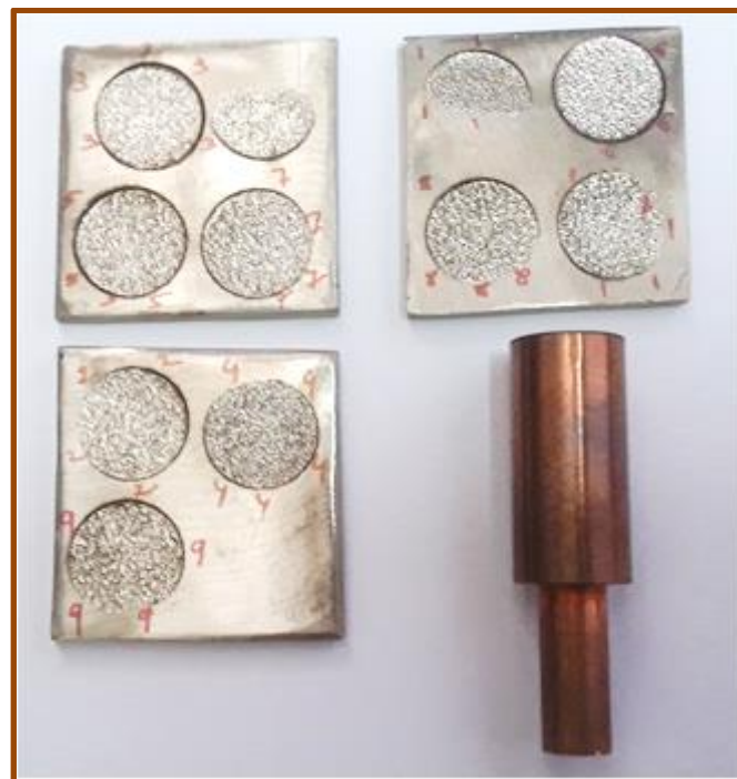
Fig. 2.3: Snapshot of EDMed work surfaces of Inconel 718 (obtained through PMEDM with SiC powder mixed kerosene as dielectric) along with copper tool electrode
