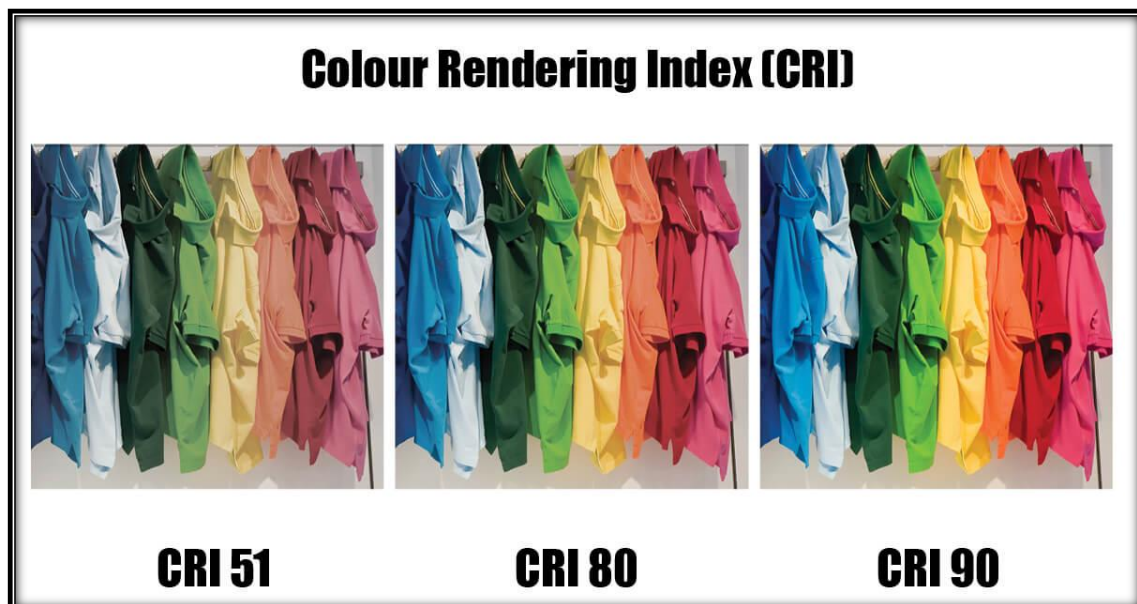
Fig 3.3.4: Effect on objects under luminaires with different levels of CRI
