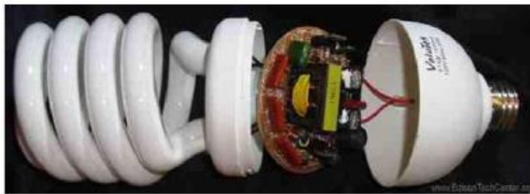
Fig 2.9: Integrated CFL lamp showing the position of Ballast inside
