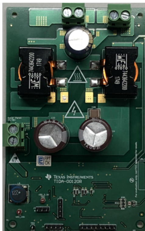
Figure 3.10: Reference Design of Solar Charge Controller
