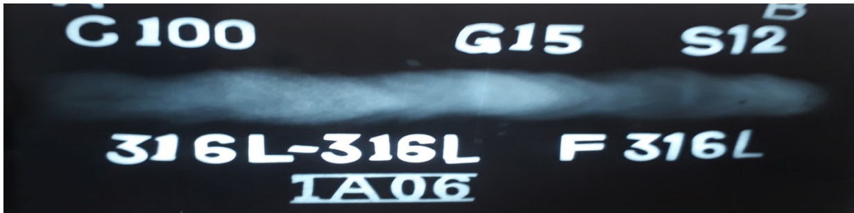
Figure 4.2 X-ray radiographic film for Sample No. S2: 316L Austenitic stainless steel as per RSM design of experiment
