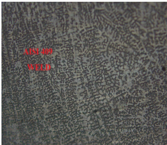
Figure 4.232 Metallographic view of Sample No. S4C: 316L Austenitic stainless steel to 409 Ferritic stainless steel (x500)
