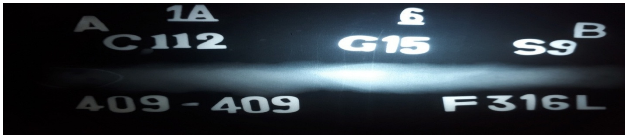
Figure 4.120 X-ray radiographic film for Sample No. S19B: 409 Ferritic stainless steel as per RSM design of experiment
