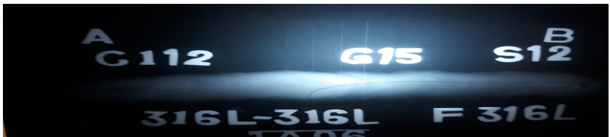
Figure 4.9 X-ray radiographic film for Sample No. S9: 316L Austenitic stainless steel as per RSM design of experiment
