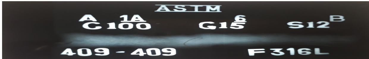
Figure 4.103 X-ray radiographic film for Sample No. S2B: 409Ferritic stainless steel as per RSM design of experiment
