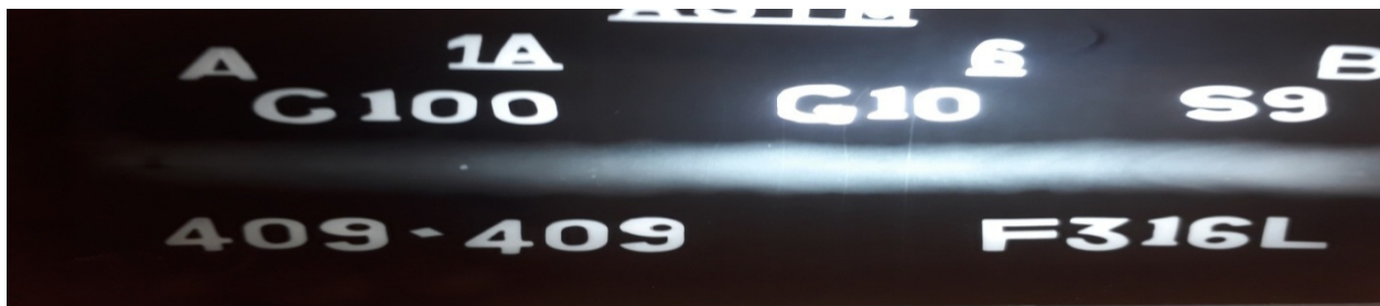
Figure 4.105 X-ray radiographic film for Sample No. S4B: 409 Ferritic stainless steel as per RSM design of experiment
