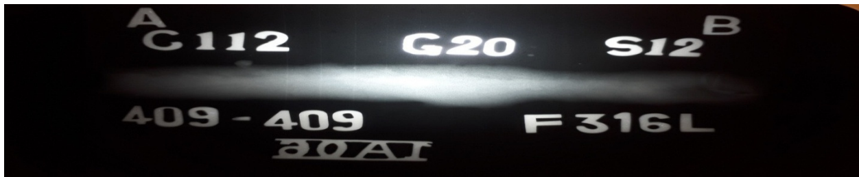
Figure 4.119 X-ray radiographic film for Sample No. S18B: 409 Ferritic stainless steel as per RSM design of experiment
