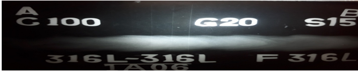
Figure 4.86 X-ray radiographic film for Sample No. S3A:316L Austenitic stainless steel as per L9 Taguchi orthogonal array design of experiment
