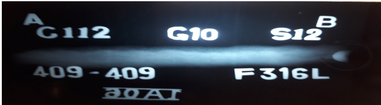
Figure 4.109 X-ray radiographic film for Sample No. S8B: 409Ferritic Stainless Steel as per RSM design of experiment
