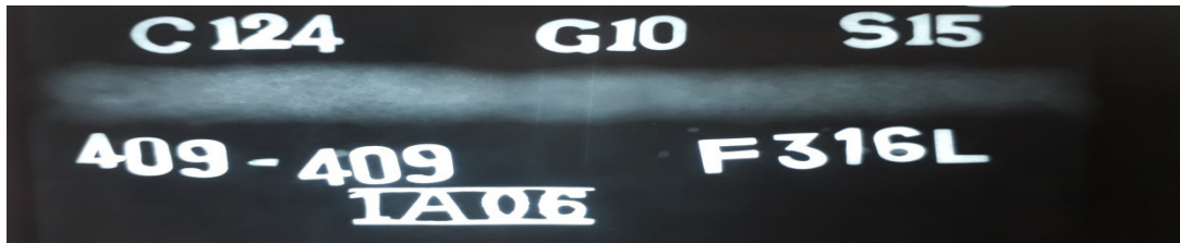
Figure 4.190 X-ray radiographic film for Sample No. S7D: 409 Ferritic Stainless Steel as L9 Taguchi orthogonal array design of experiment
