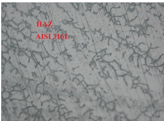
Figure 4.233 Metallographic view of Sample No. S5C: 316L Austenitic stainless steel to 409 Ferritic stainless steel (x500)
