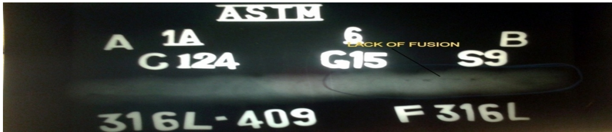
Figure 4.209 X-ray radiographic film for Sample No.S8C: 316L Austenitic to 409 Ferritic stainless steel as per L9 Taguchi orthogonal array design of experiment
