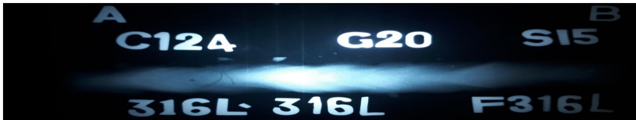
Figure 4.13 X-ray radiographic film for Sample No. S13: 316L Austenitic stainless steel as per RSM design of experiment
