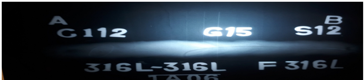
Figure 4.17 X-ray radiographic film for Sample No. S17: 316L Austenitic stainless steel as per RSM design of experiment
