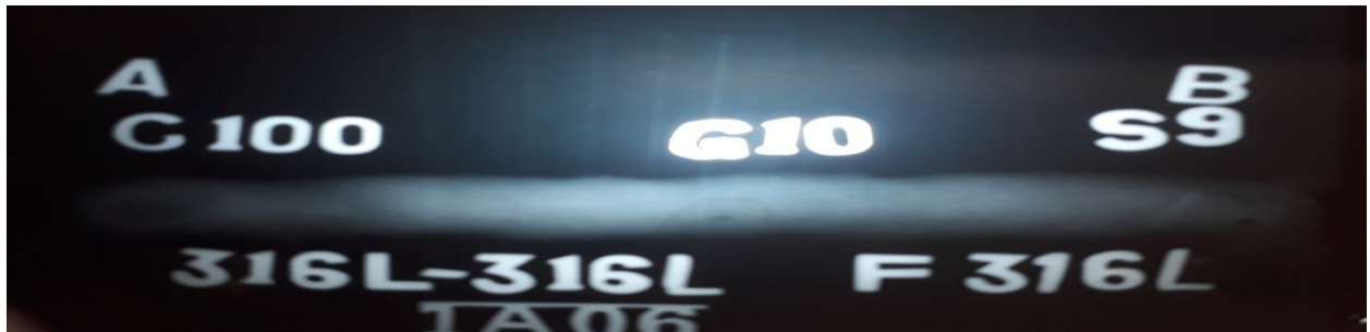
Figure 4.4 X-ray radiographic film for Sample No. S4: 316L Austenitic stainless steel as per RSM design of experiment
