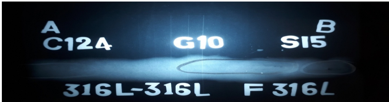
Figure 4.14 X-ray radiographic film for Sample No. S14: 316L Austenitic stainless steel as per RSM design of experiment
