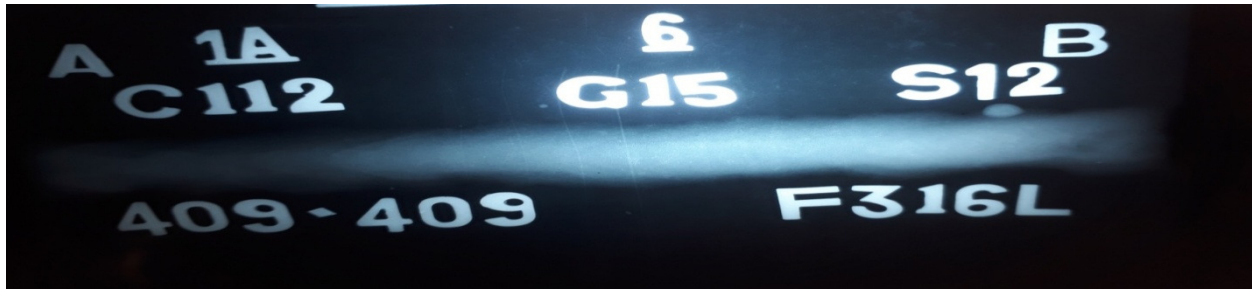
Figure 4.117 X-ray radiographic film for Sample no. S16B: 409 Ferritic stainless steel as per RSM design of experiment
