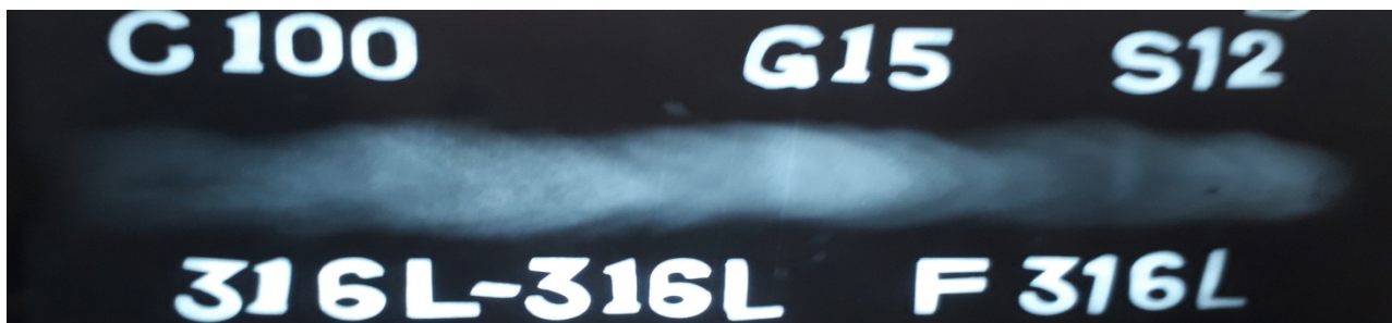
Figure 4.85 X-ray radiographic film for Sample No. S2A: 316L Austenitic stainless steel as per L9 Taguchi orthogonal array design of experiment
