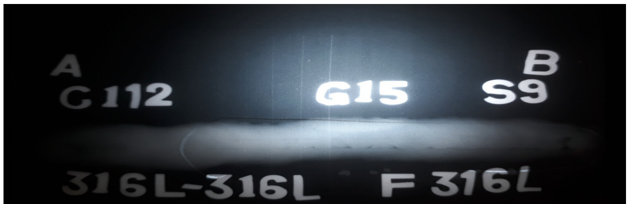
Figure 4.19 X-ray radiographic film for Sample No. S19: 316L Austenitic stainless steel as per RSM design of experiment
