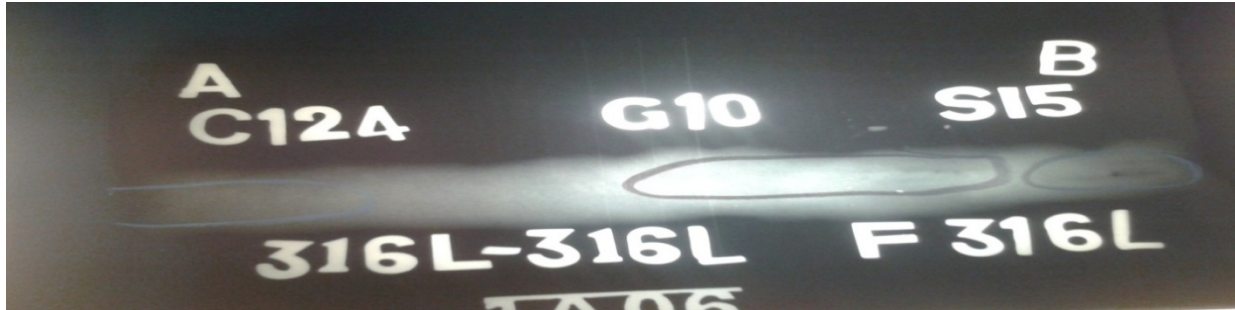
Figure 4.90 X-ray radiographic film for Sample No. S7A:316L Austenitic stainless steel as per L9 Taguchi orthogonal array design of experiment
