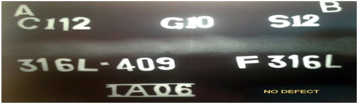
Figure 4.205 X-ray radiographic film for Sample No. S4C: 316L Austenitic to 409 Ferritic stainless steel as per L9 Taguchi orthogonal array design of experiment
