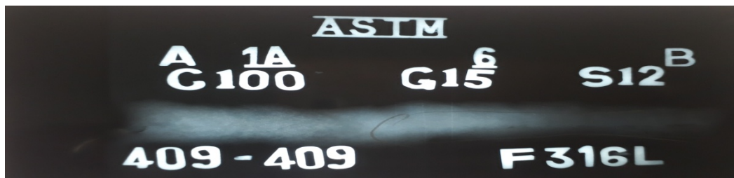
Figure 4.185 X-ray radiographic film for Sample No. S2D: 409 Ferritic Stainless Steel as L9 Taguchi orthogonal array design of experiment
