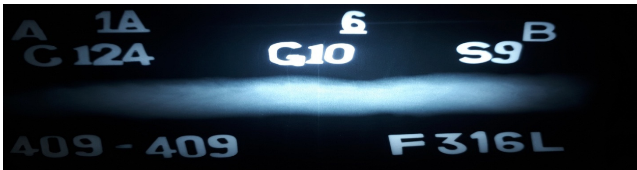
Figure 4.111 X-ray radiographic film for Sample No. S10B: 409 Ferritic stainless steel as per RSM design of experiment
