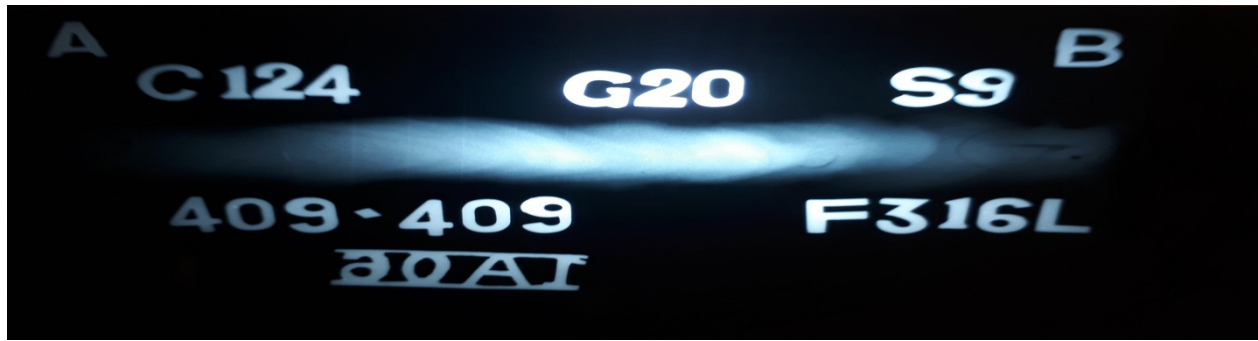
Figure 4.121 X-ray radiographic film for Sample no. S20B: 409 Ferritic stainless steel as per RSM design of experiment
