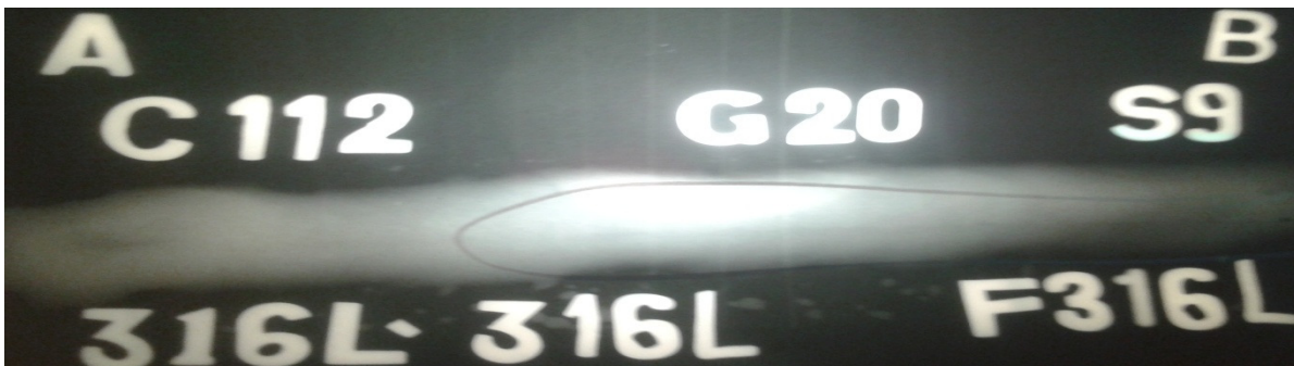
Figure 4.89 X-ray radiographic film for Sample No. S6A:316L Austenitic stainless steel as per L9 Taguchi orthogonal array design of experiment
