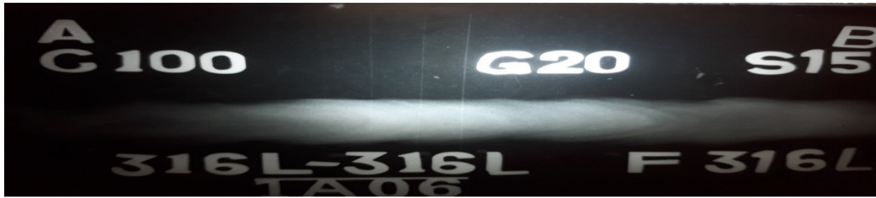
Figure 4.6 X-ray radiographic film for Sample No. S6: 316L Austenitic stainless steel as per RSM design of experiment
