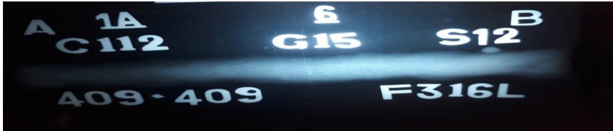
Figure 4.102 X-ray radiographic film for Sample No. S1B: 409Ferritic stainless steel as per RSM design of experiment
