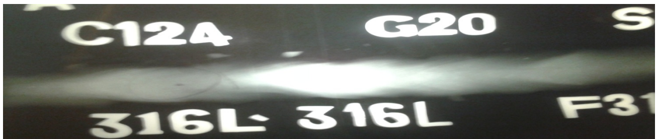
Figure 4.20 X-ray radiographic film for Sample No. S20: 316L Austenitic stainless steel as per RSM design of experiment
