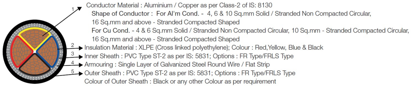
Figure 4.5: Cross Sectional View of Selected LT Cable
