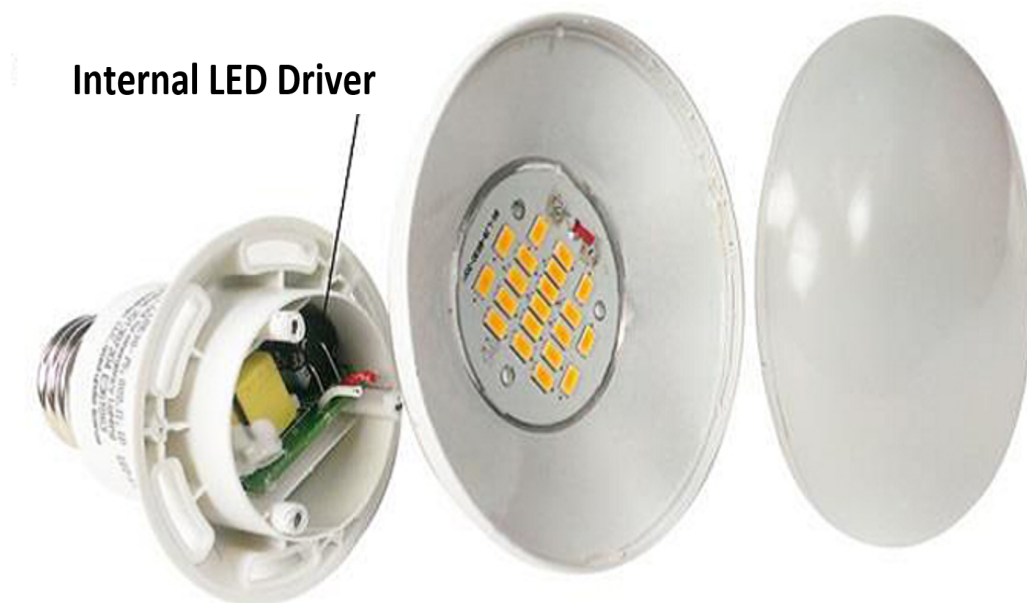
Figure 1: Internal LED Driver in a LED Bulb [1]
