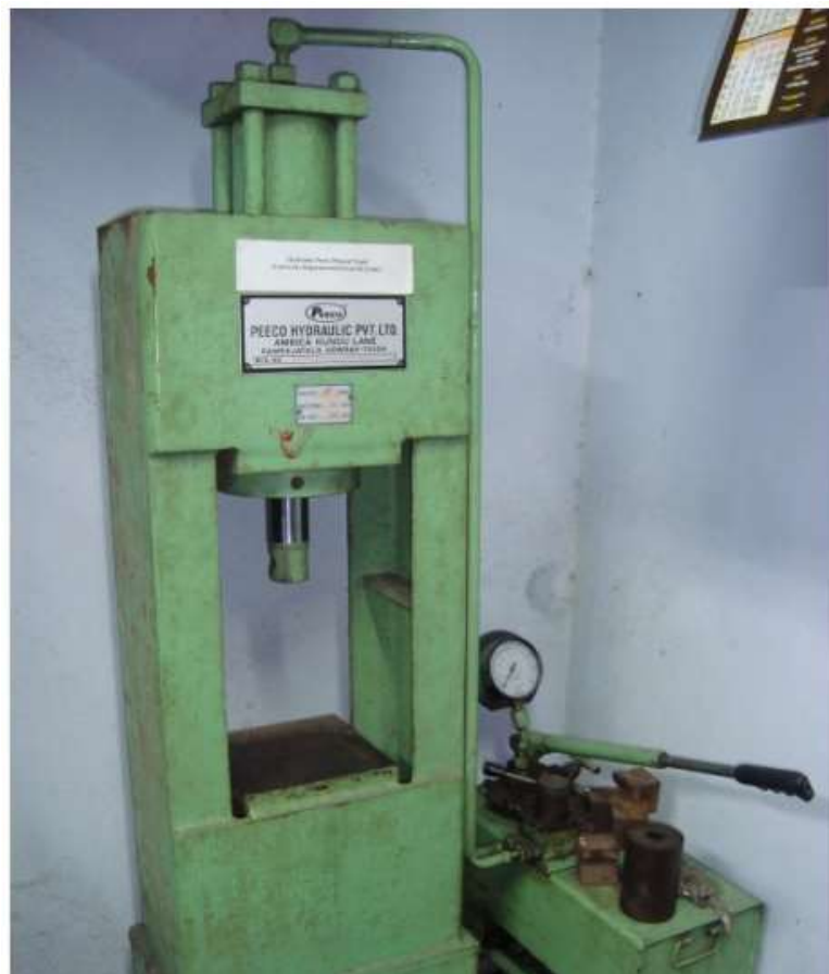
Figure 3.20: 20 Ton Hydraulic Press used for upsetting of MMC specimens at room temperature.
