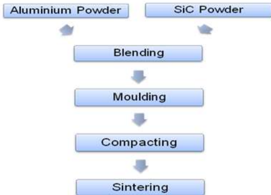
Figure 3.3: Various steps involved in synthesis of Al-SiCp composites in P/M technique.
