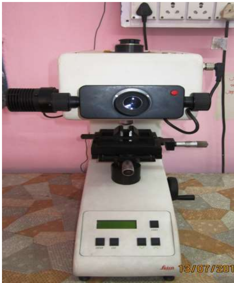
Figure 3.15: The micro hardness testing machine, for measuring micro hardness of MMCs.
