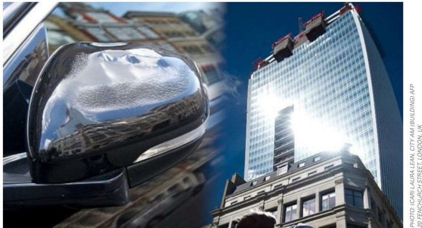
Fig 6.09 concentrated reflected sunlight deformed a car mirror
