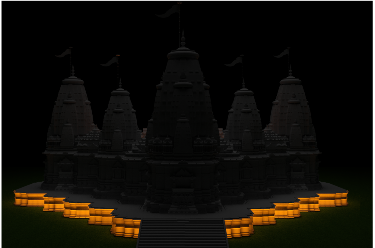
Figure 40: Above image is a screenshot taken in the 3DS Max Software after Rendering (This is the front side of the temple) Corner Profile of 1800K CCT is used
