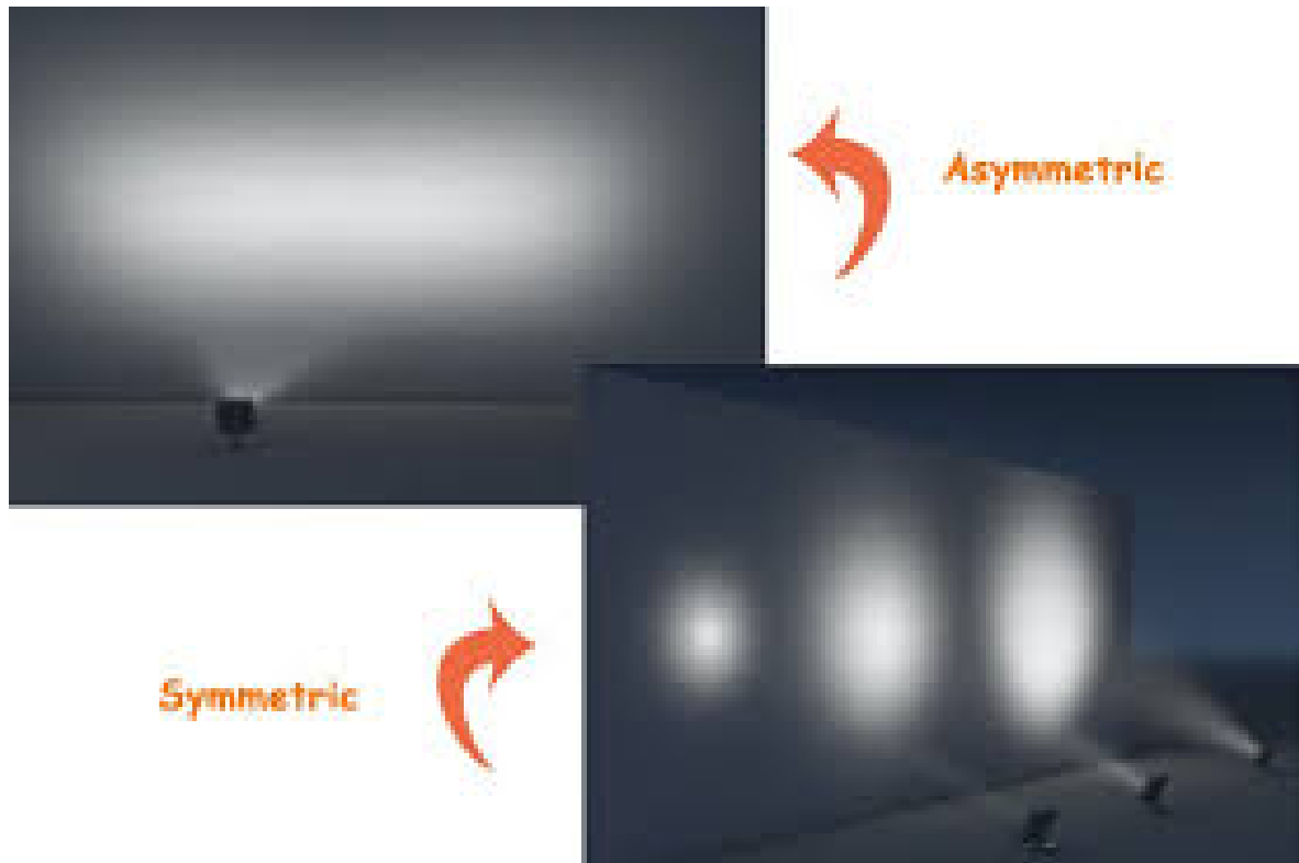
Figure 24: Difference between symmetrical or asymmetrical beam angle wash lights
