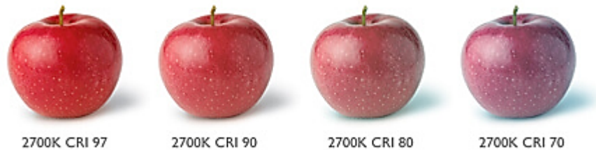
Figure 19: Difference between low CRI & high CRI lighting
