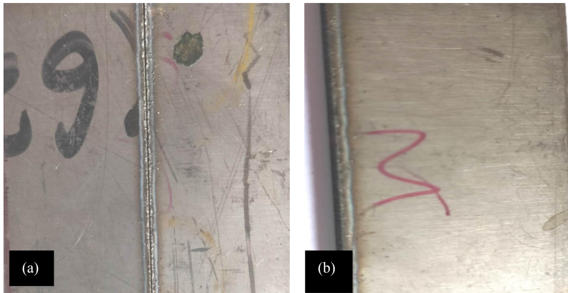
Fig. 5.3 Photographic view of the workpiece cut with laser
