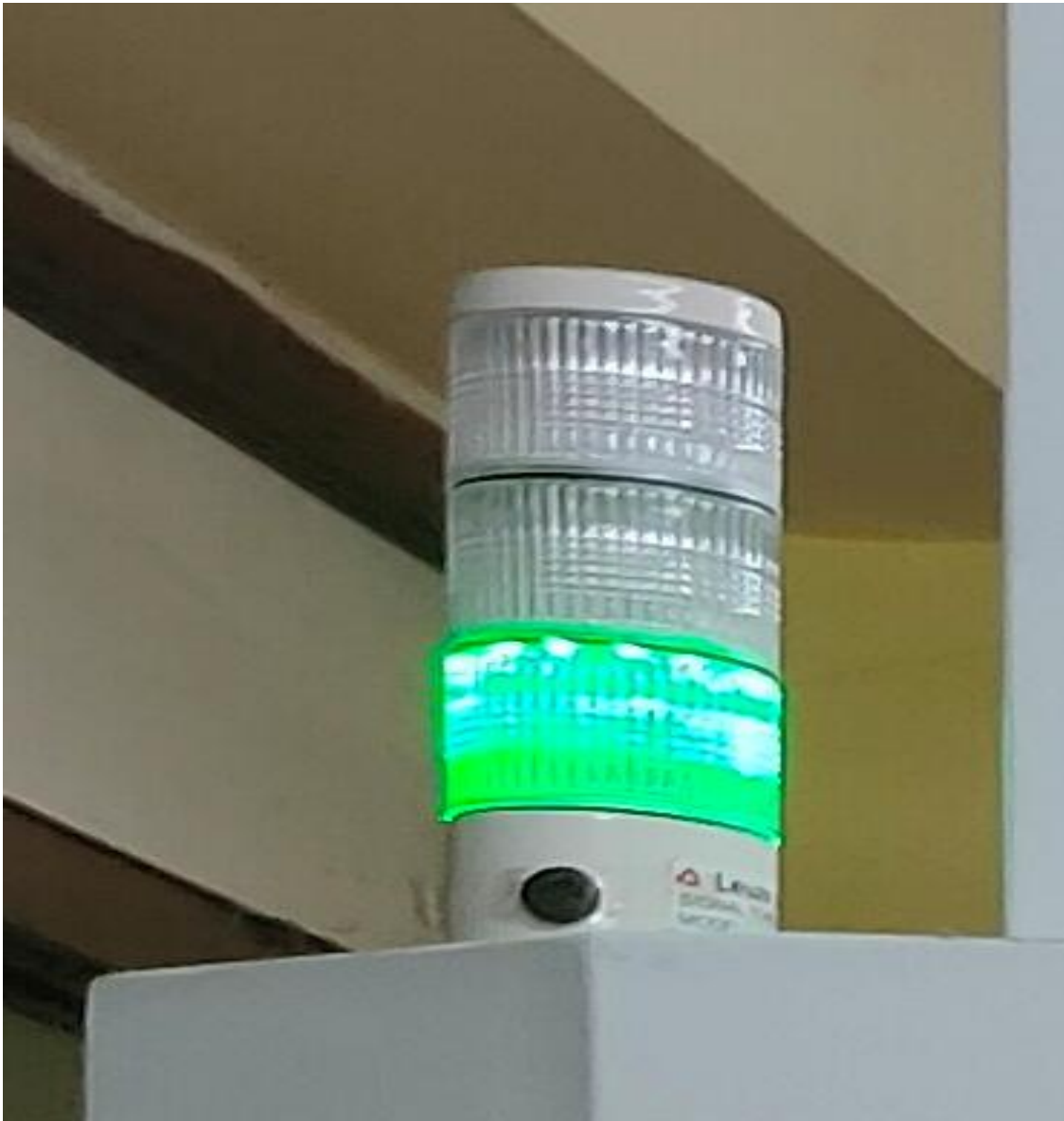
Fig. 3.10 Indicator lamps mounted on the top of the workspace, currently glowing in green symbolizing the machine is ready for operation
