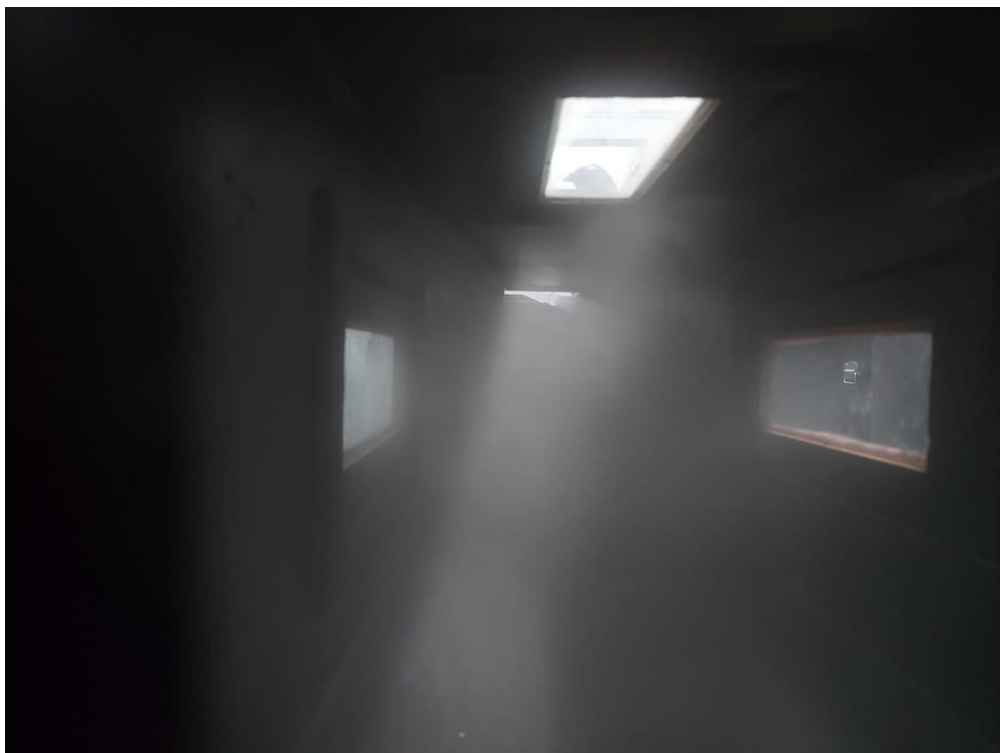
Fig.5.10. Natural fog (Type VI) inside the wooden box
