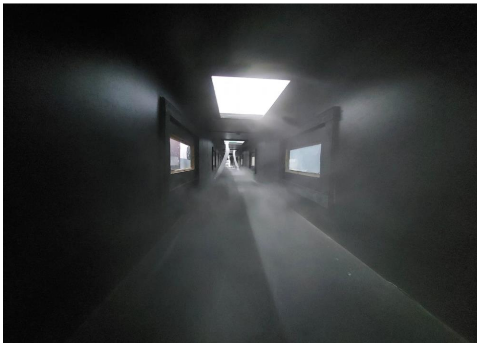
Fig.5.6. Natural fog (Type II) inside the wooden box
