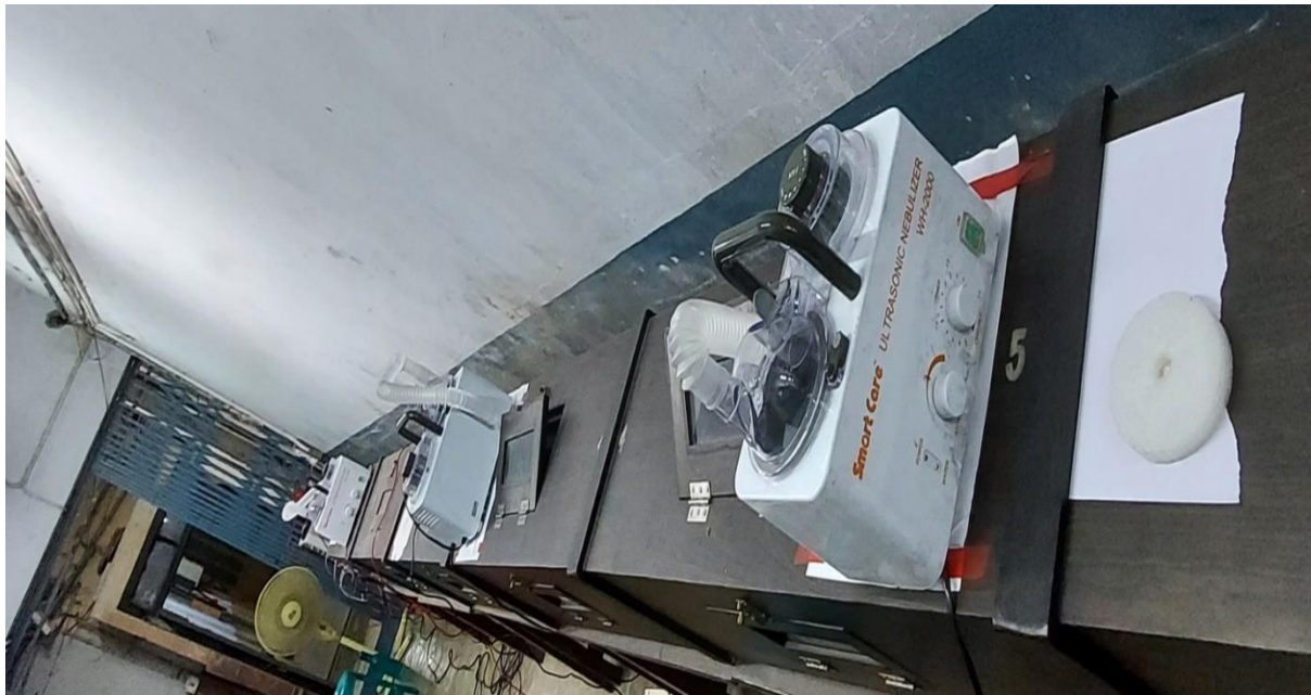
Fig.5.4. Artificial fog simulation setup with ultrasonic nebulizers
