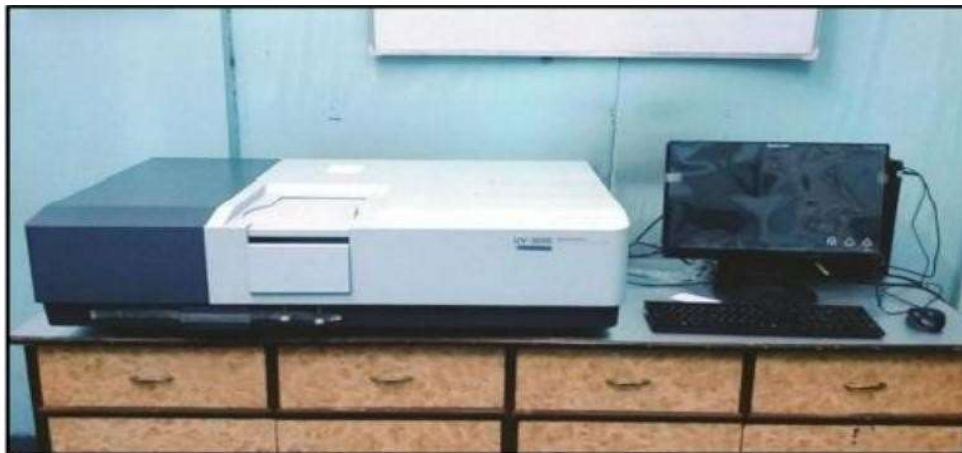
Figure 7.29: UV-VIS-NIS (SHIMADZU UV-3600) Spectrophotometer
