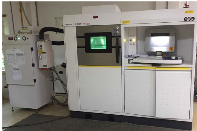
Figure 17: EOS direct metal laser sintering machine (model: EOSINT-M280) installed at Central Tool Room and Training Center, Bhubaneswar, Odisha.
