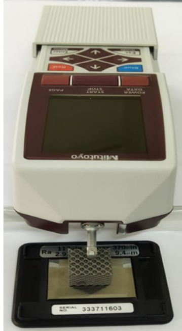
Figure 24. Talysurf surface roughness tester (Mitutoyo SJ-210).
