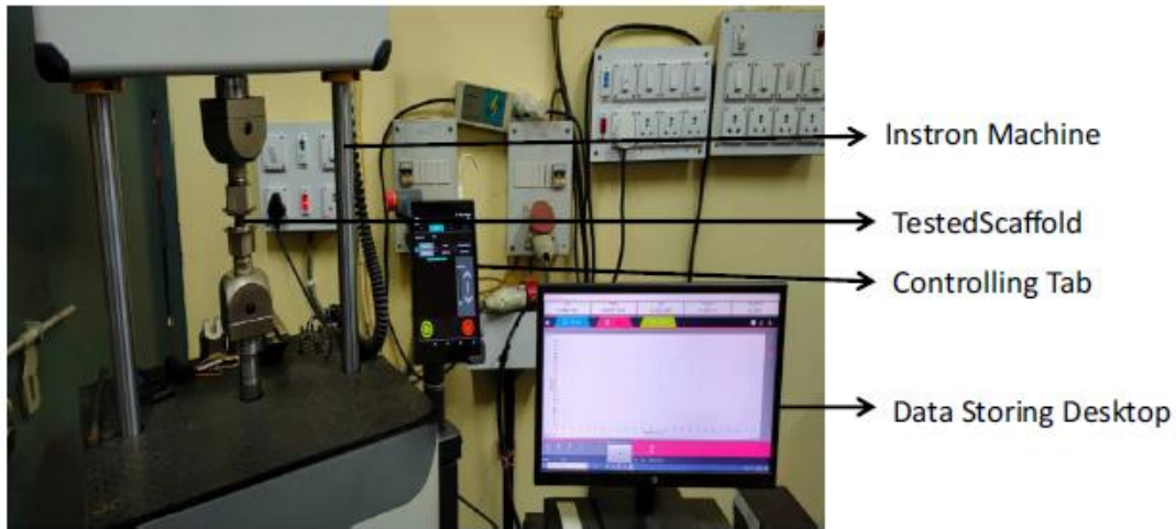
Figure 27: Experimental setup for compression test on INSTRON.
