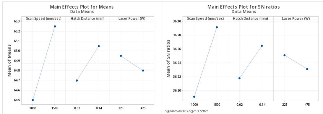
Figure 34: Main Effects Plots for Means and SN Ratios for Vinties.
