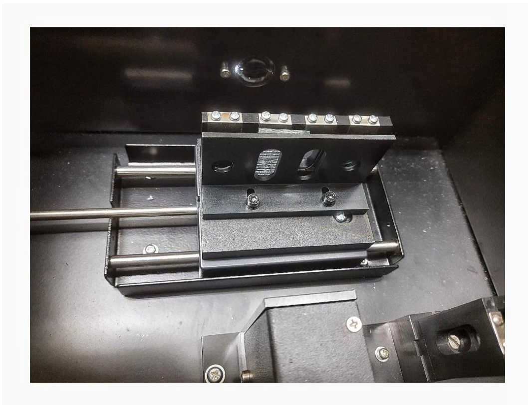
Fig 3.2 Experimentation of Textured FTO Coated Glass in Spectrophotometer.
