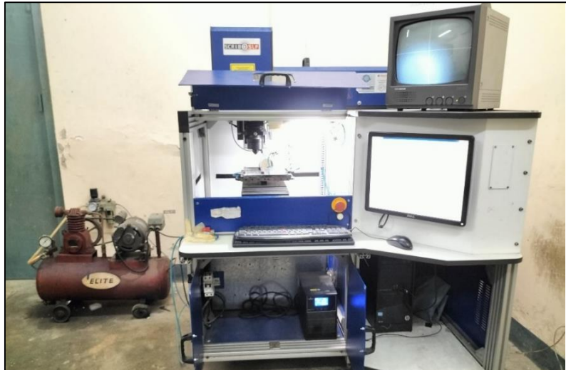
Fig.3.2. Diode Pump Fiber Laser Marking machine in Operational mode.
