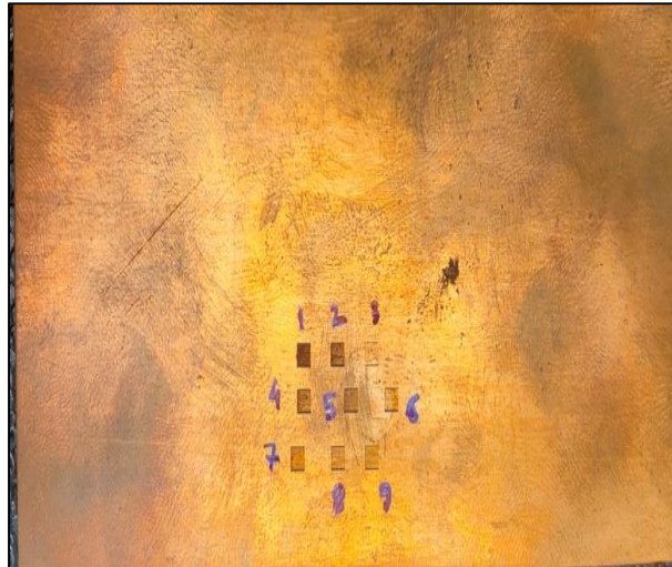
Fig. 5.2. Laser marked Beryllium Copper sample comprising a total of 9 squares.
