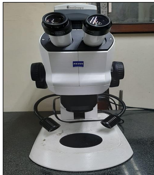
Fig 5.3. ZEISS STEMI 508 optical microscope used for HAZ measurement.
