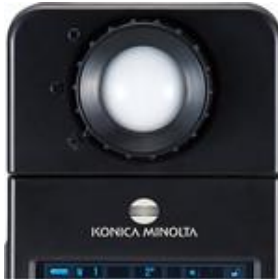
Fig 8.5 Zero Adjustment Without receptor Cap
