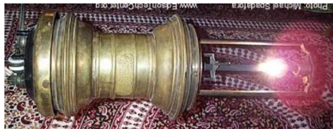
Fig 3.2 : A lit arc lamp from the 1880s as was used in urban lighting and factories.
