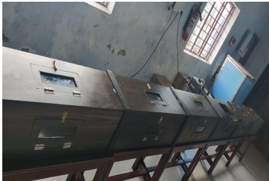
Fig 3.14: Actual figure of the artificial fog simulation box/chamber
