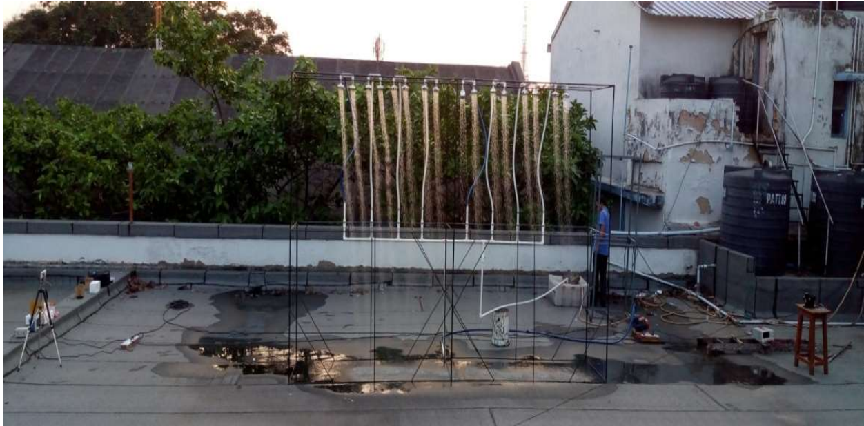
Fig 3.10 . The rain simulation setup
