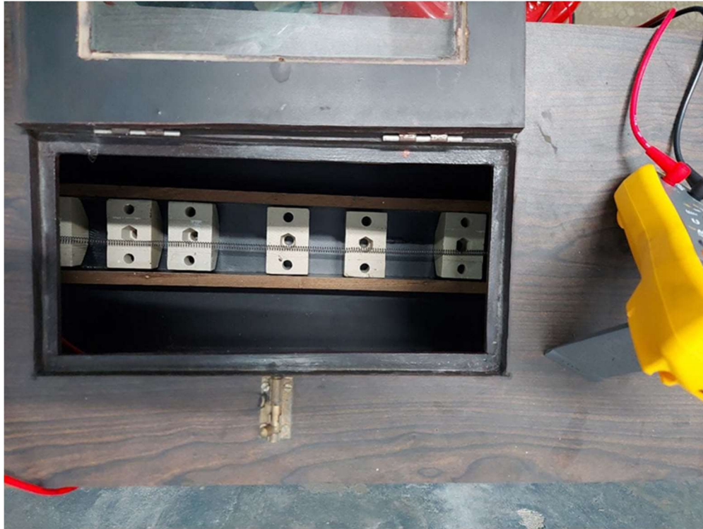
Fig 3.17: Coils are put on the ceramic pots
