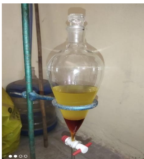
Fig 3.6: Separation of crude biodiesel and glycerol
