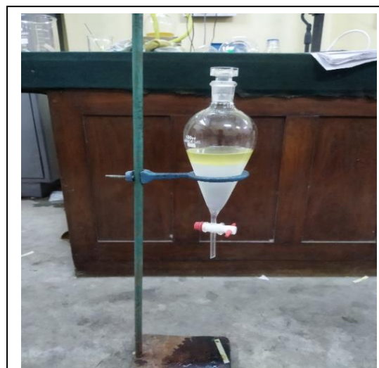
Fig 3.8: Separation of biodiesel and water after purification
