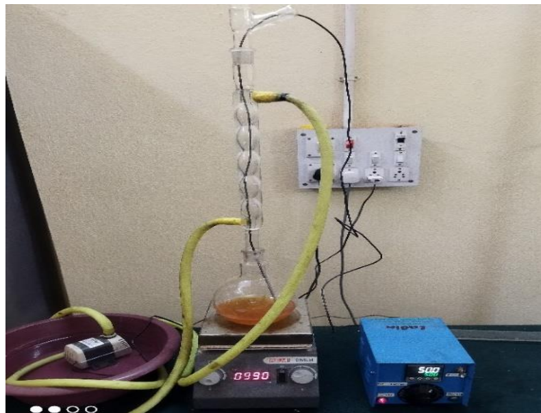
Fig 3.5: Setup of Transesterification process of WSO/CSO
