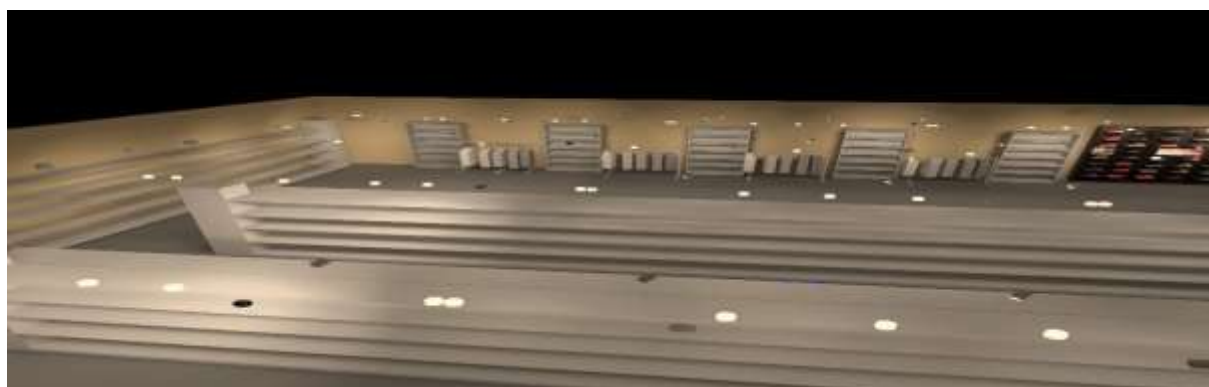
Fig. No.16: contrast (2 to1) on clothing racks and shoe racks for customer impression
