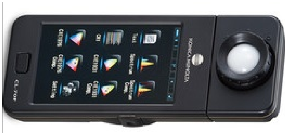
Figure 47: CRI Illuminance Meter CL-70F
