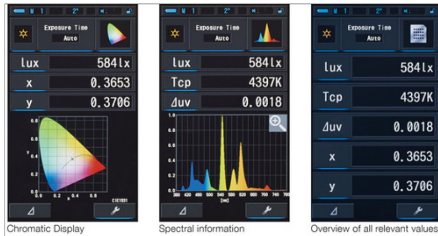
Figure 49: Chromaticity Diagram (for CCT Calculation), Spectral Composition & Others important Information
