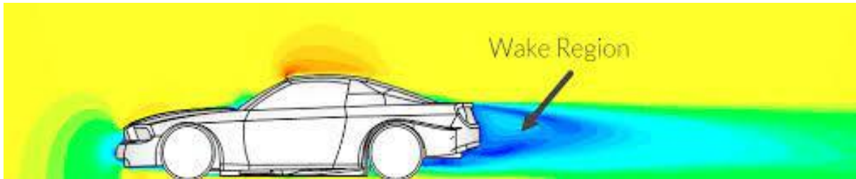
Figure 1.3- formation of wake region and flow separation
