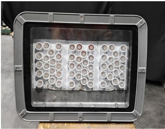
Fig.6.10. (a) 90W Monochromatic amber LED luminaire
