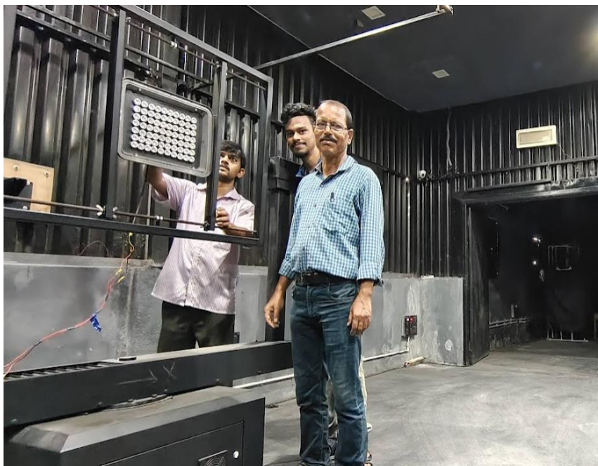
Fig.6.4. (a) Goniophotometer Experimental setup [Puspasish Mal (me), Samir Mandi (lab assistant) and Pradip Pal (lab assistant) in frame]
