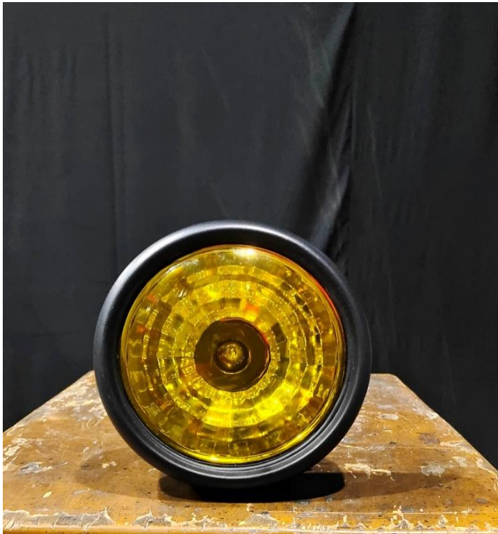
Fig.6.19. (a) Currently used railway fog lamp with halogen bulb luminaire
