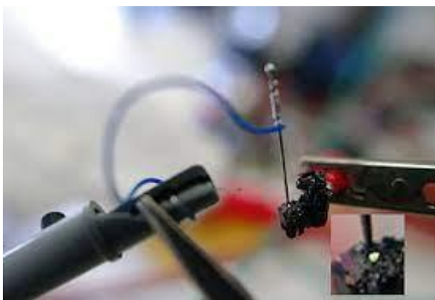
Fig.4.2.(a) contact on crystal SiCcreates H. Round's original experiment (Source-Wikipedia.org)
