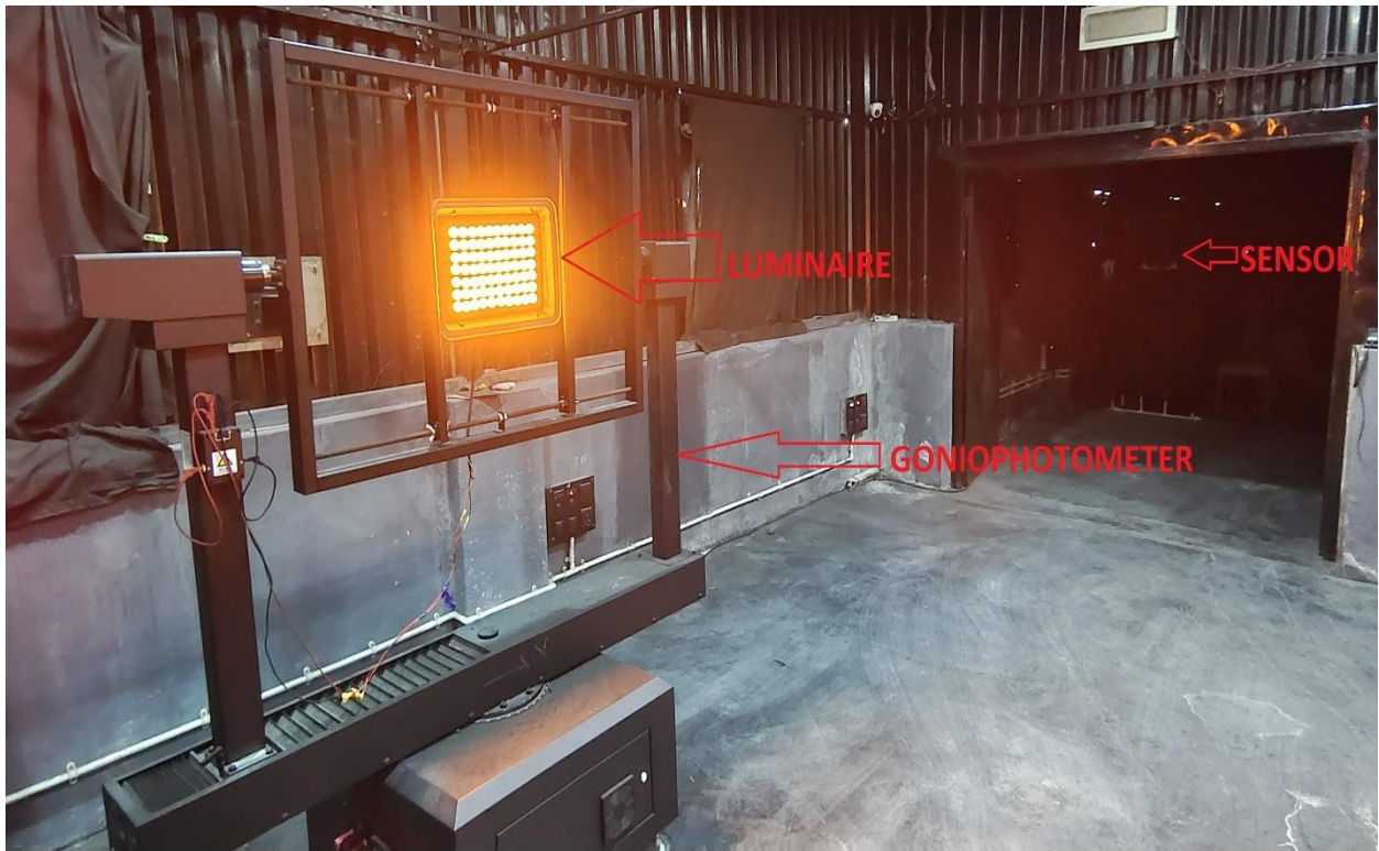
Fig.6.4.(b) Goniophotometer experimental setup showing luminaire and light sensor in our JADAVPUR UNIVERSITY ILLUMINATION Laboratory
