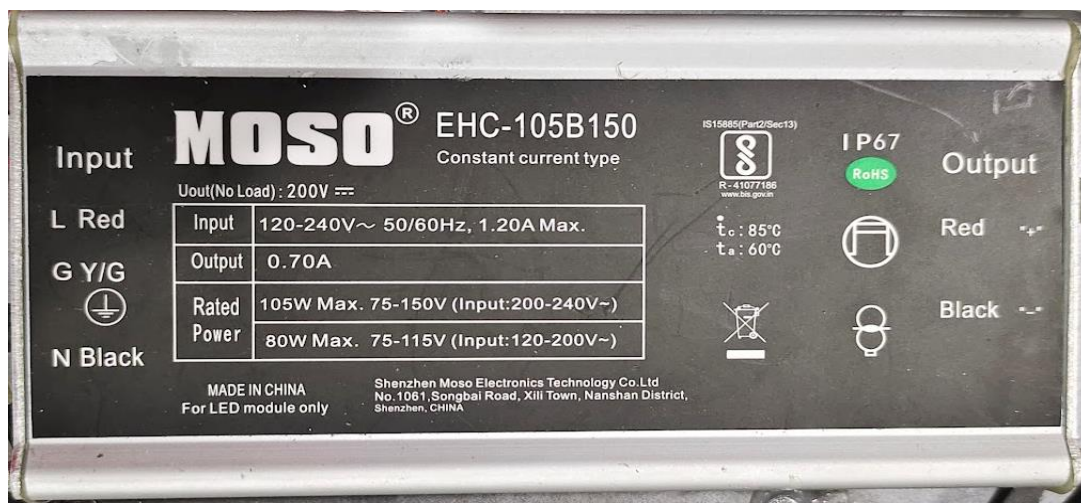
Fig.4.14. Constant current LED driver
