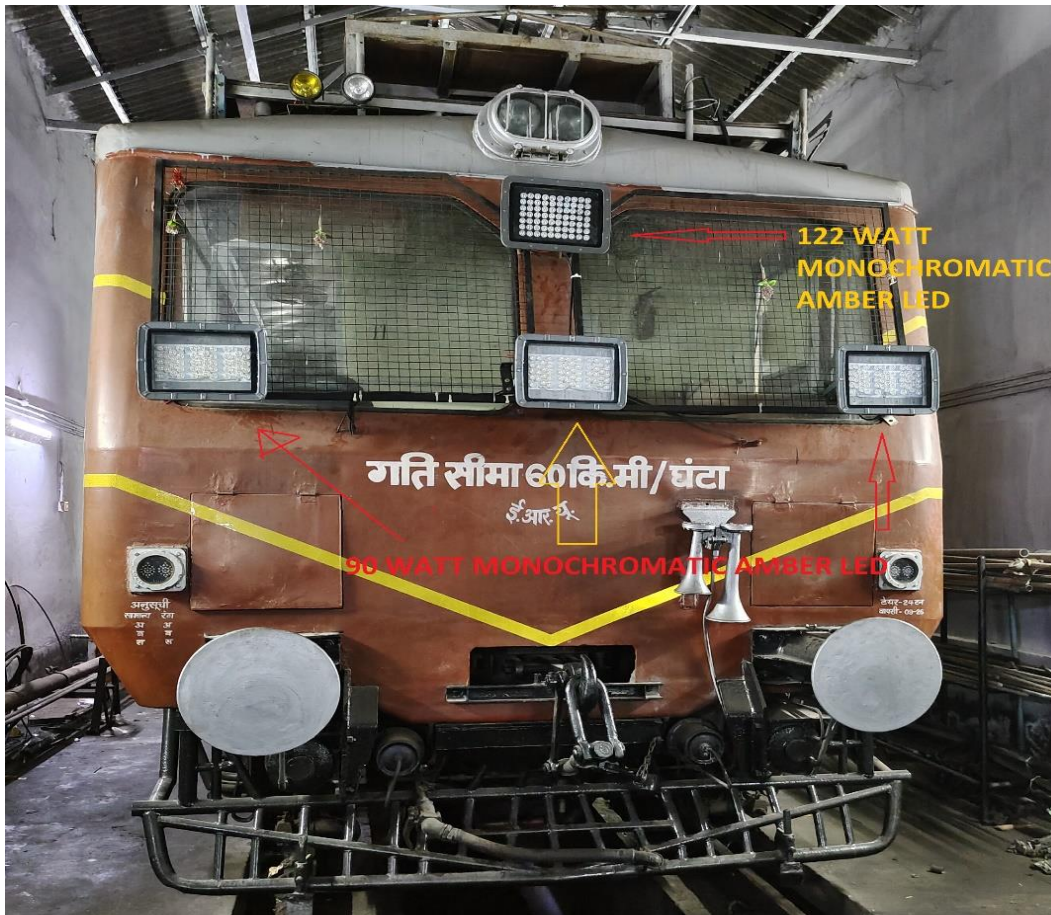
Fig.6.28. (a) Railway tower van with fog lighting system setup consisting 4 monochromatic amber LED luminaires
