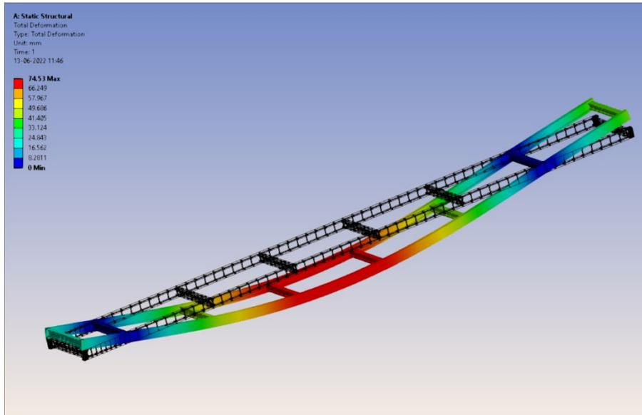
**Figure 4.1 Deformation due to static loading**
