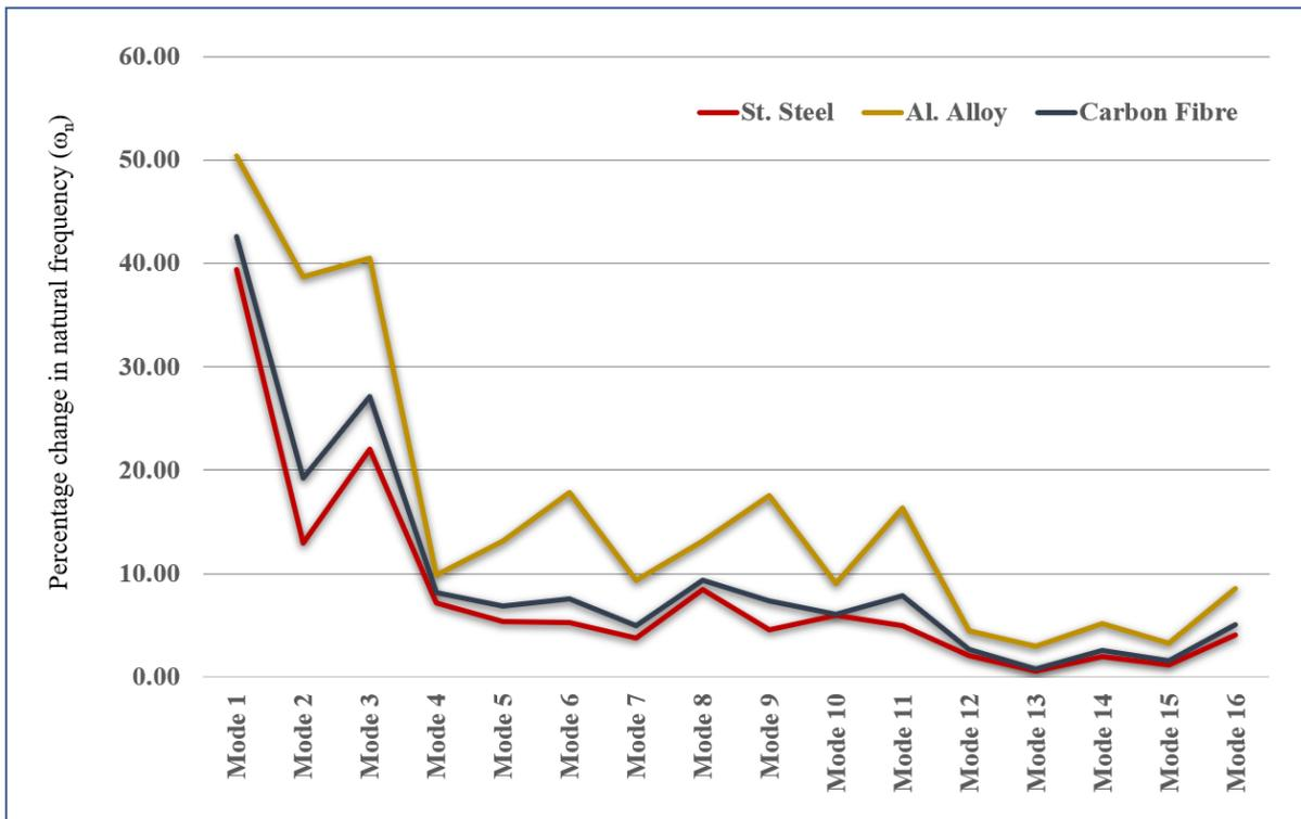
**Figure 4.3 Percentage change between load pre-stressed and load free modes in all three materials**
