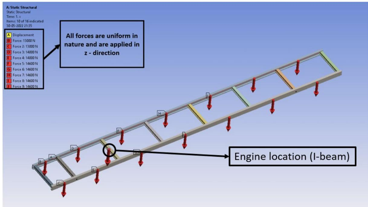
**Figure 3.4 Distribution of The Loads on The Chassis**
