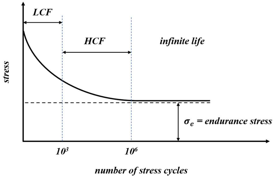
**Figure 1.1 S-N curve for fatigue failure**
