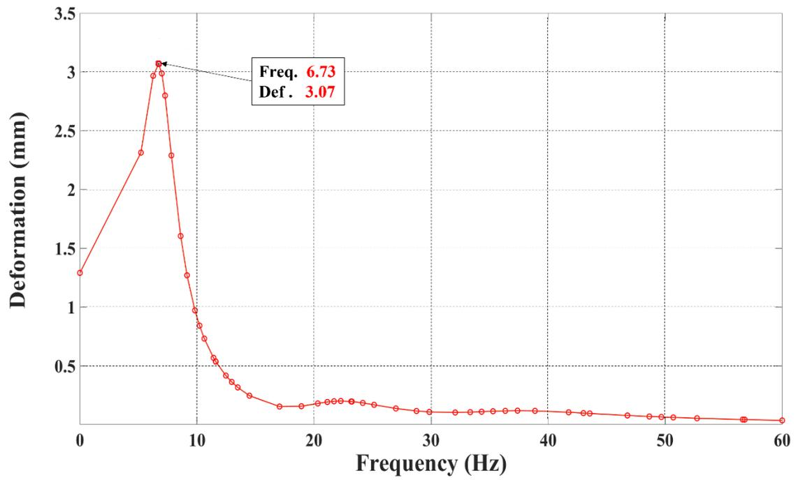
*Figure 4.6 Deformation vs Frequency for load free chassis*
