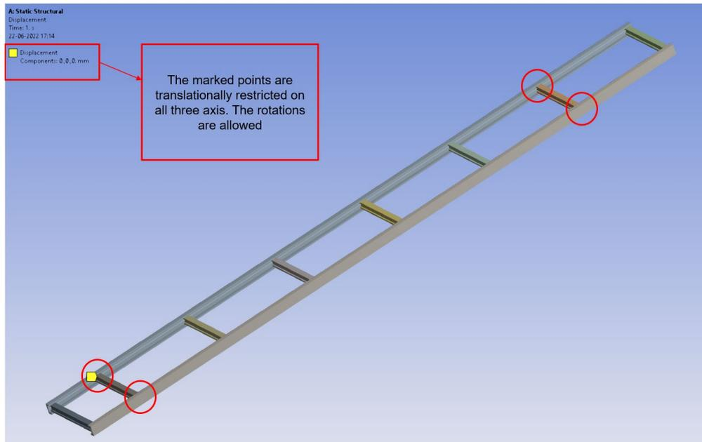
**Figure 3.5 Boundary Conditions of The Model**
