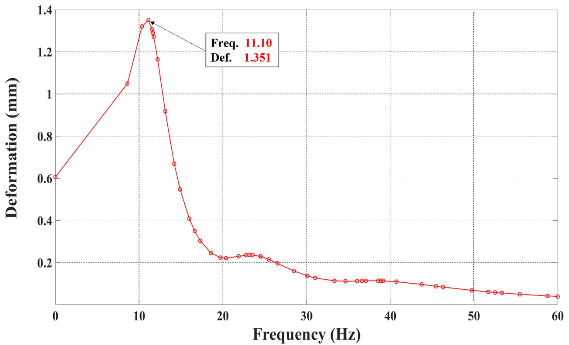
*Figure 4.7 Deformation vs Frequency for pre-stressed chassis*
