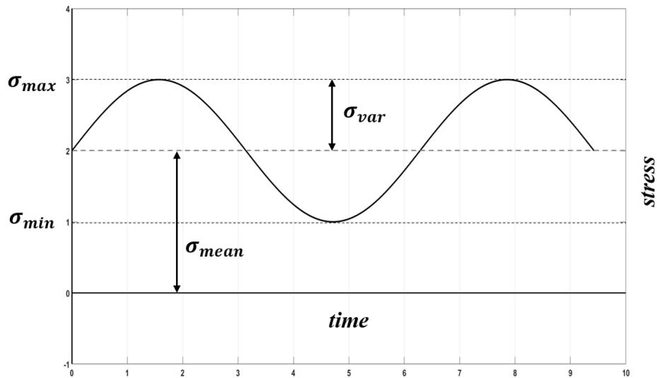
**Figure 1.2** Cyclic loading showing different stress parameter for fatigue
