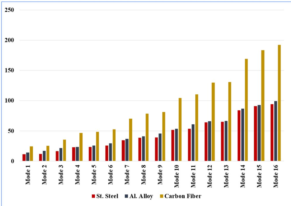
*Figure 4.5 Comparison between pre-stressed modes of all three materials*
