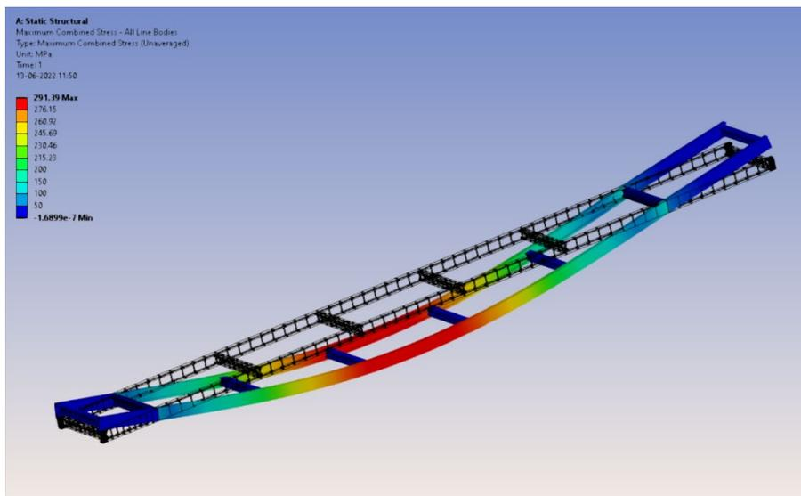
**Figure 4.2 Combined stress due to static loading**
