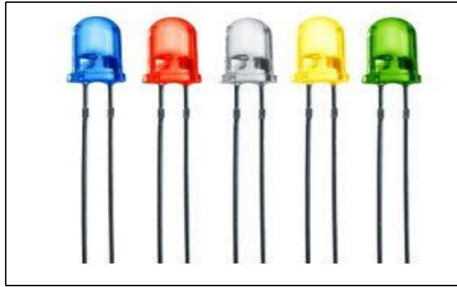
Fig. 3.1: 5 mm blue, red, white, yellow, green LEDs
