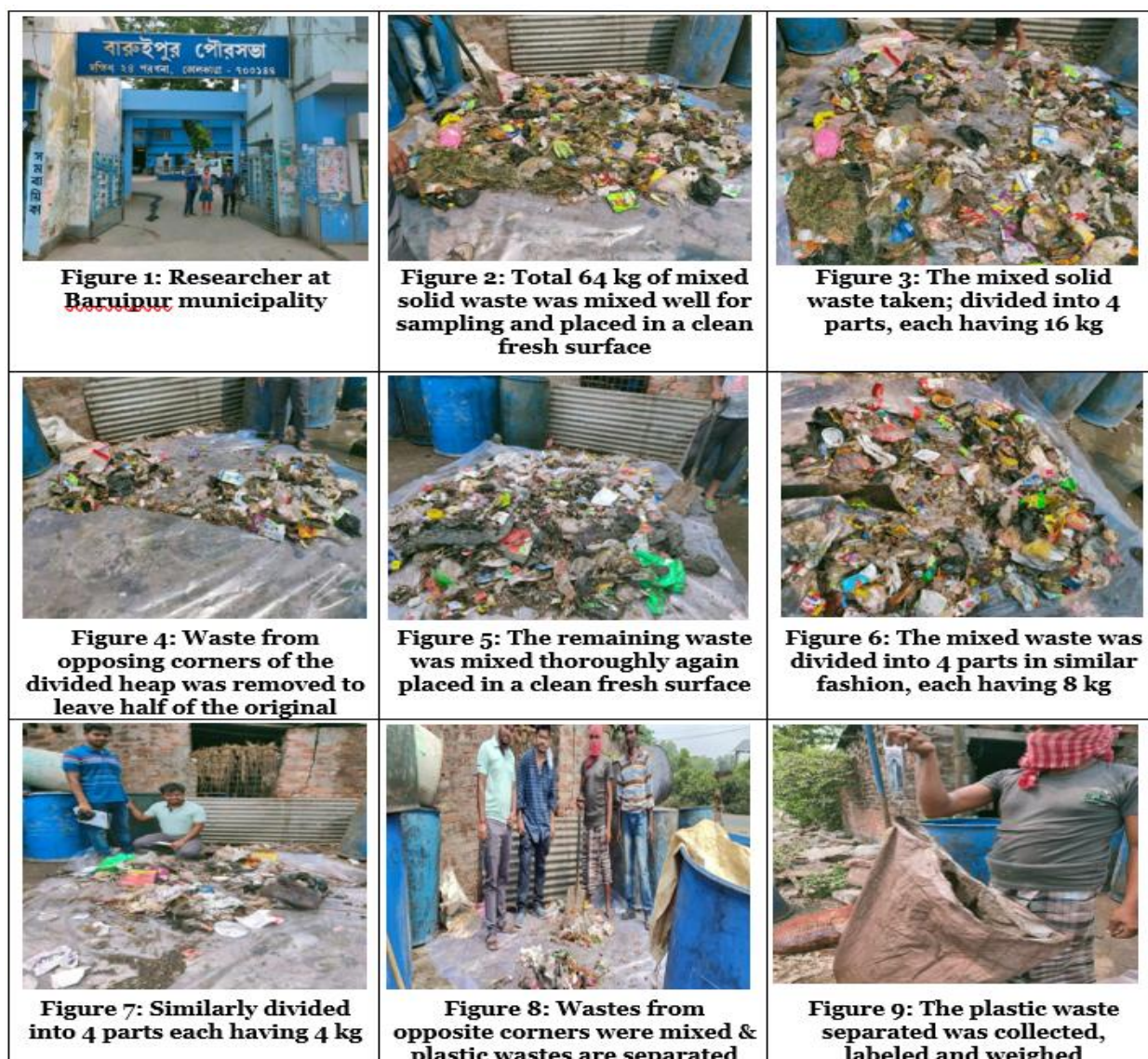
Fig. 21: Sampling Procedure of Plastic Waste at Baruipur Dumpsite
