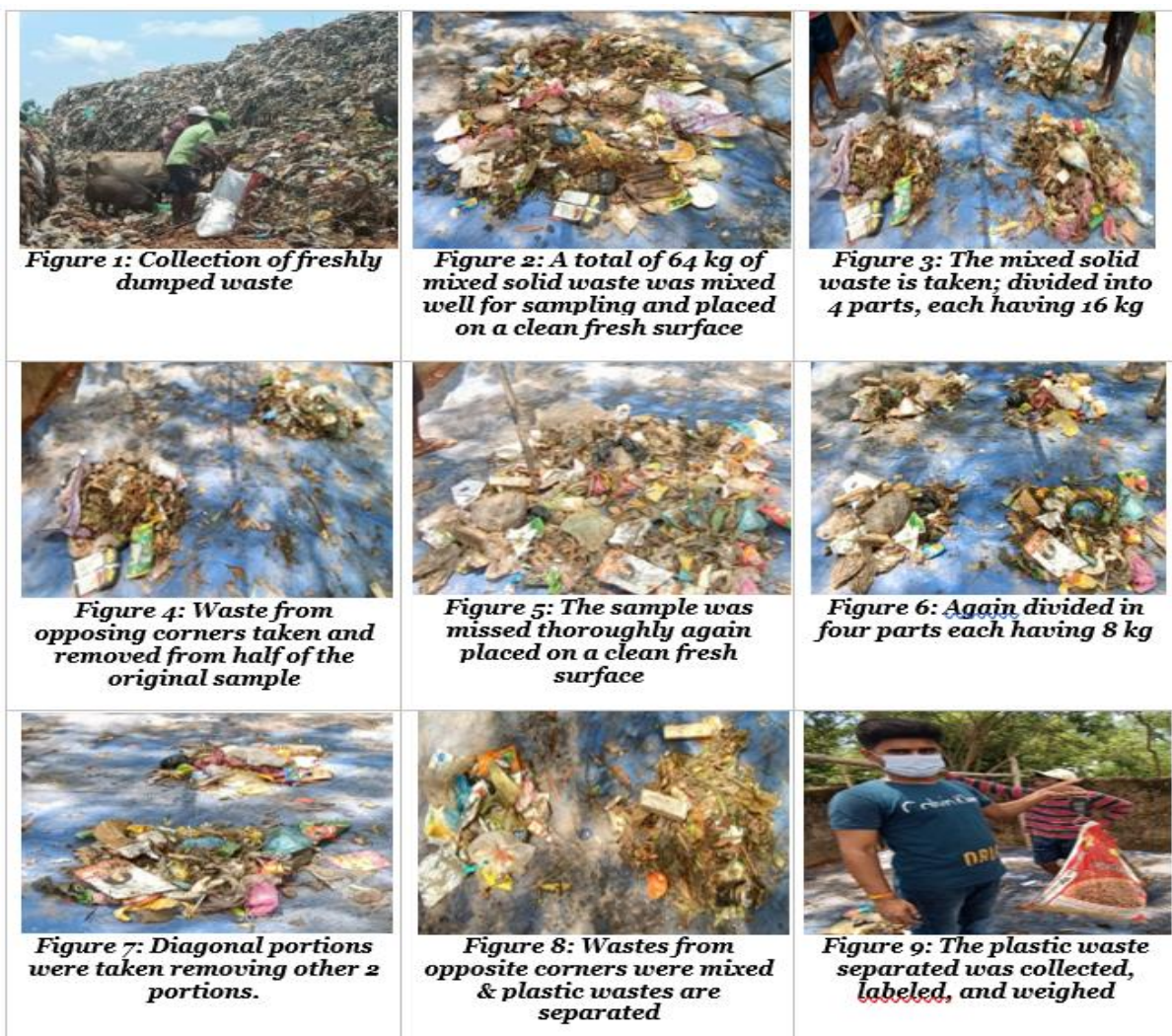
Fig. 26: Sampling Procedure of Plastic Waste Cuttack Dumpsite
