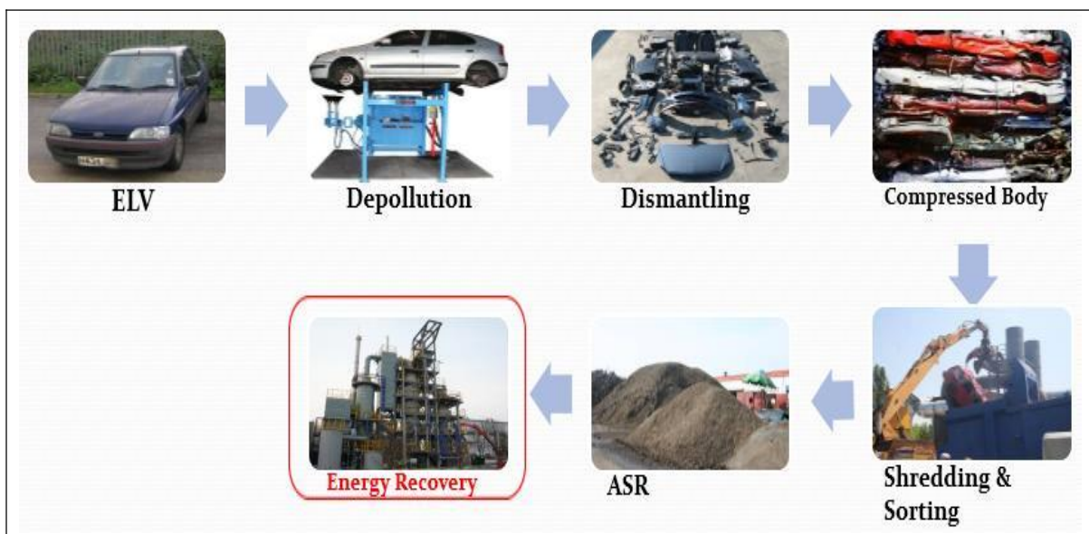
Figure 45: ELV flow from collection to final disposal in developed nations such as EU
