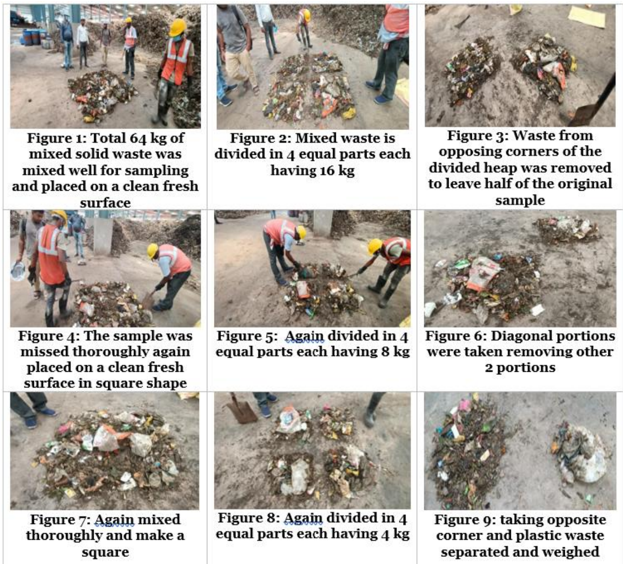
Fig. 27: Sampling Procedure of Plastic Waste Berhampur Dumpsite
