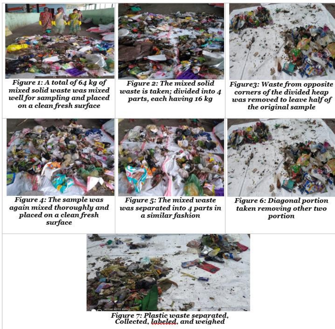
Fig. 30: Sampling Procedure of Plastic Waste Keonjhar Dumpsite
