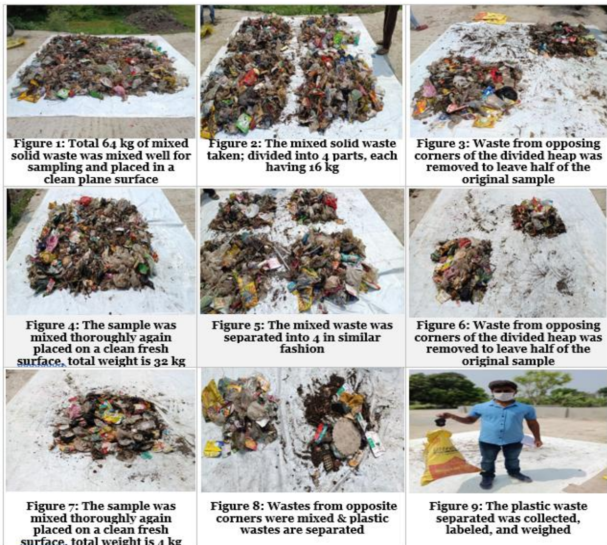
Fig.24: Sampling Procedure of Plastic Waste at Murshidabad Dumpsite
