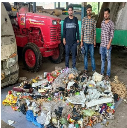
Total 64 kg of mixed solid waste was mixed well for sampling and placed in a clean fresh surface
