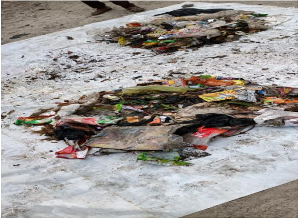
Figure 6: Waste from opposing corners of the divided heap was removed to leave half of the original sample
