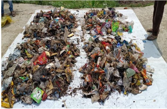
Figure 3: The mixed solid waste taken; divided into 4 parts, each having 16 kg
