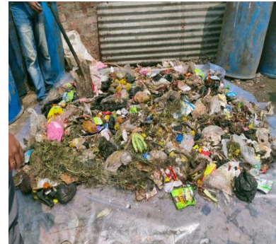
Total 64 kg of mixed solid waste was mixed well for sampling and placed in a clean fresh surface
