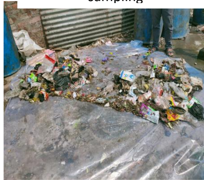
Waste from opposing corners of the divided heap was removed to leave half of the original sample
