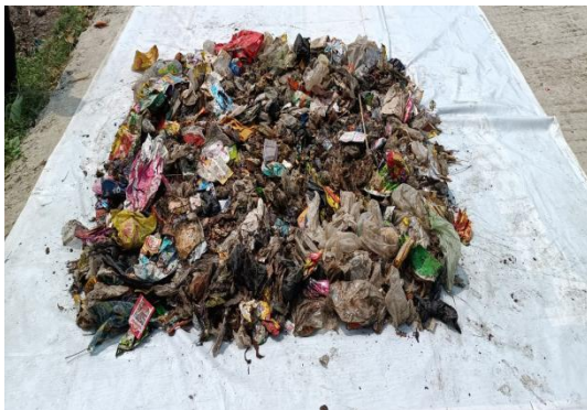
Figure 5: The sample was mixed thoroughly again placed in a clean fresh surface, total weight is 32 kg
