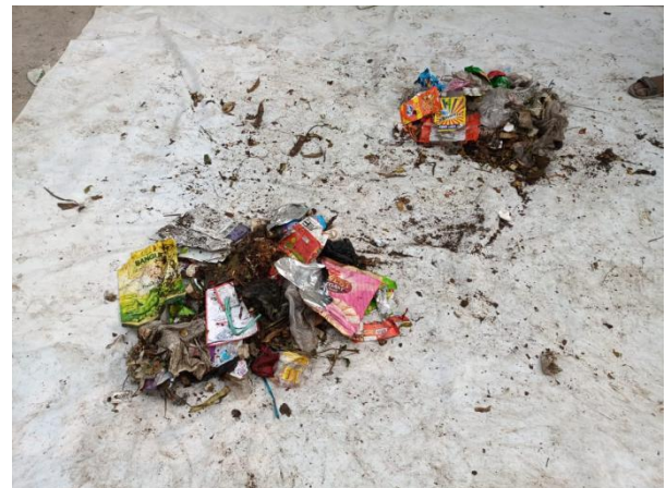
Figure 12: Waste from opposing corners of the divided heap was removed to leave half of the original sample
