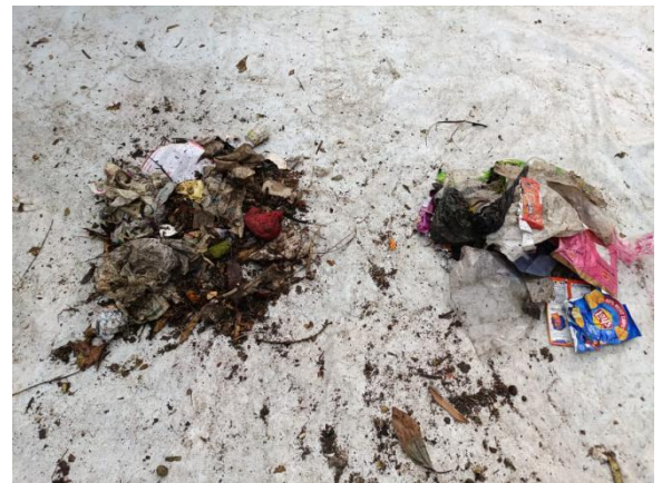
Figure 15: Wastes from opposite corners were mixed & plastic wastes are separated
