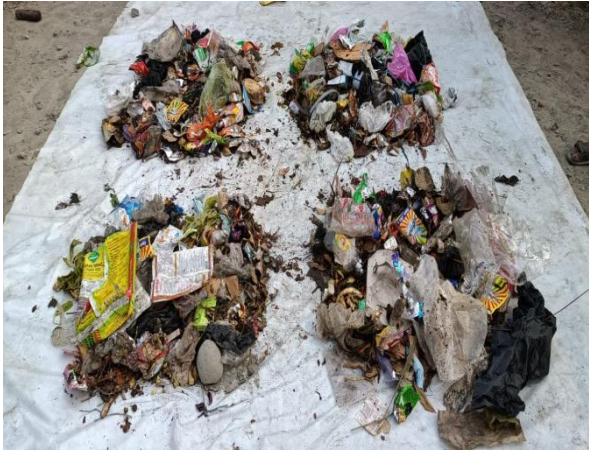
Figure 5: The mixed solid waste taken; divided into 4 parts, each having 16 kg
