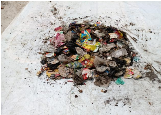
Figure 11: The sample was mixed thoroughly again placed in a clean fresh surface, total weight is 8 kg
