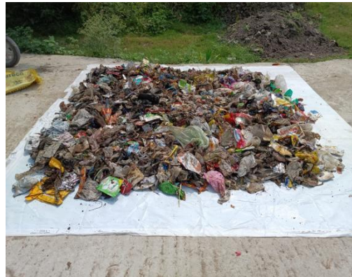
Figure 2: Total 64 kg of mixed solid waste was mixed well for sampling and placed in a clean plane surface
