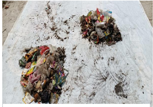
Figure 10: Waste from opposing corners of the divided heap was removed to leave half of the original
