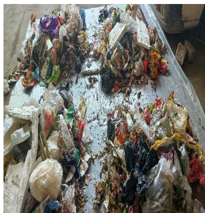
The mixed solid waste taken; divided into 4 parts, each having 16 kg
