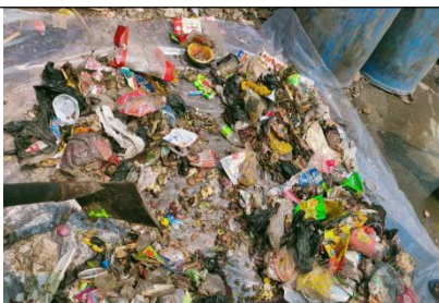
The mixed waste was divided into 4 parts in similar fashion, each having 8 kg
