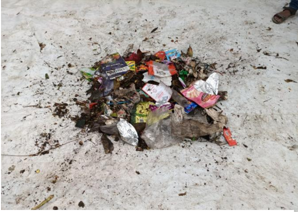
Figure 13: The sample was mixed thoroughly again placed in a clean fresh surface, total weight is 8 kg
