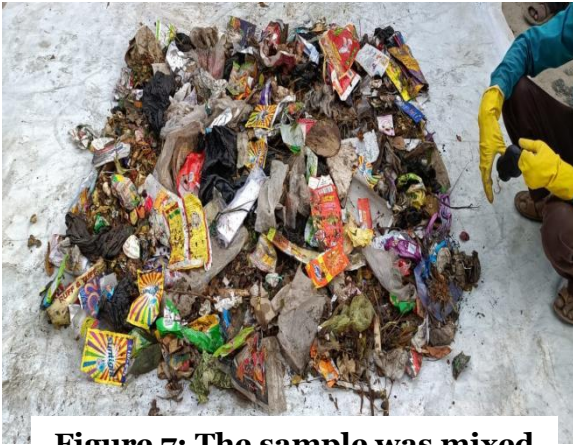
Figure 7: The sample was mixed thoroughly again placed in a clean fresh surface, total weight is 32 kg
