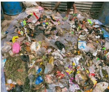
The mixed solid waste taken divided into 4 parts having each 16 kg
