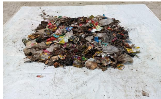
Figure 8: The sample was mixed thoroughly again placed in a clean fresh surface, total weight is 16 kg
