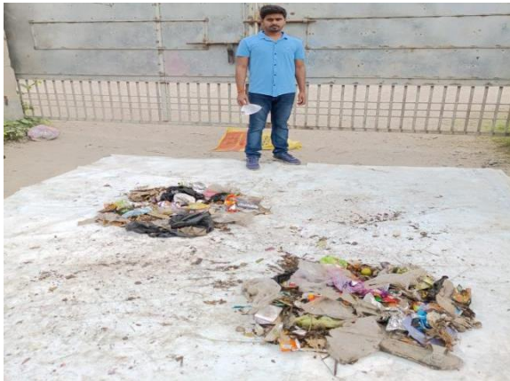
Figure 9: Waste from opposing corners of the divided heap was removed to leave half of the original sample
