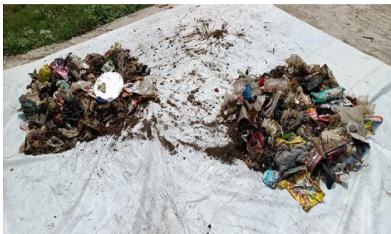
Figure 7: Waste from opposing corners of the divided heap was removed to leave half of the original sample
