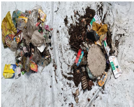
Figure 13: Wastes from opposite corners were mixed & plastic wastes are separated
