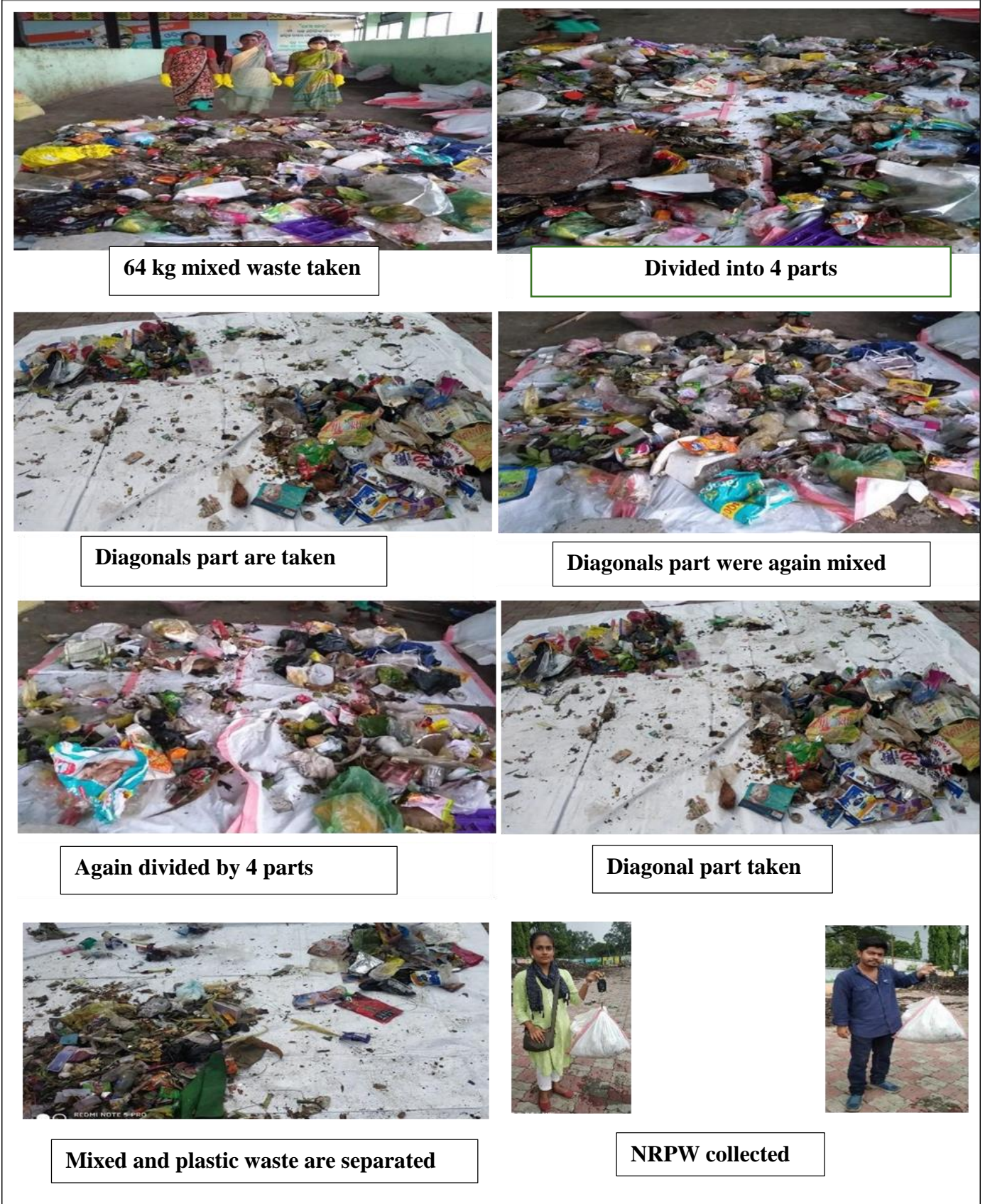
Figure 30: Sampling Procedure of Plastic Waste on Keonjhar Dumpsite
