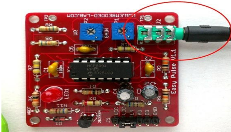
Fig No: (24) HRM-2511E connection with Easy Pulse Sensor
