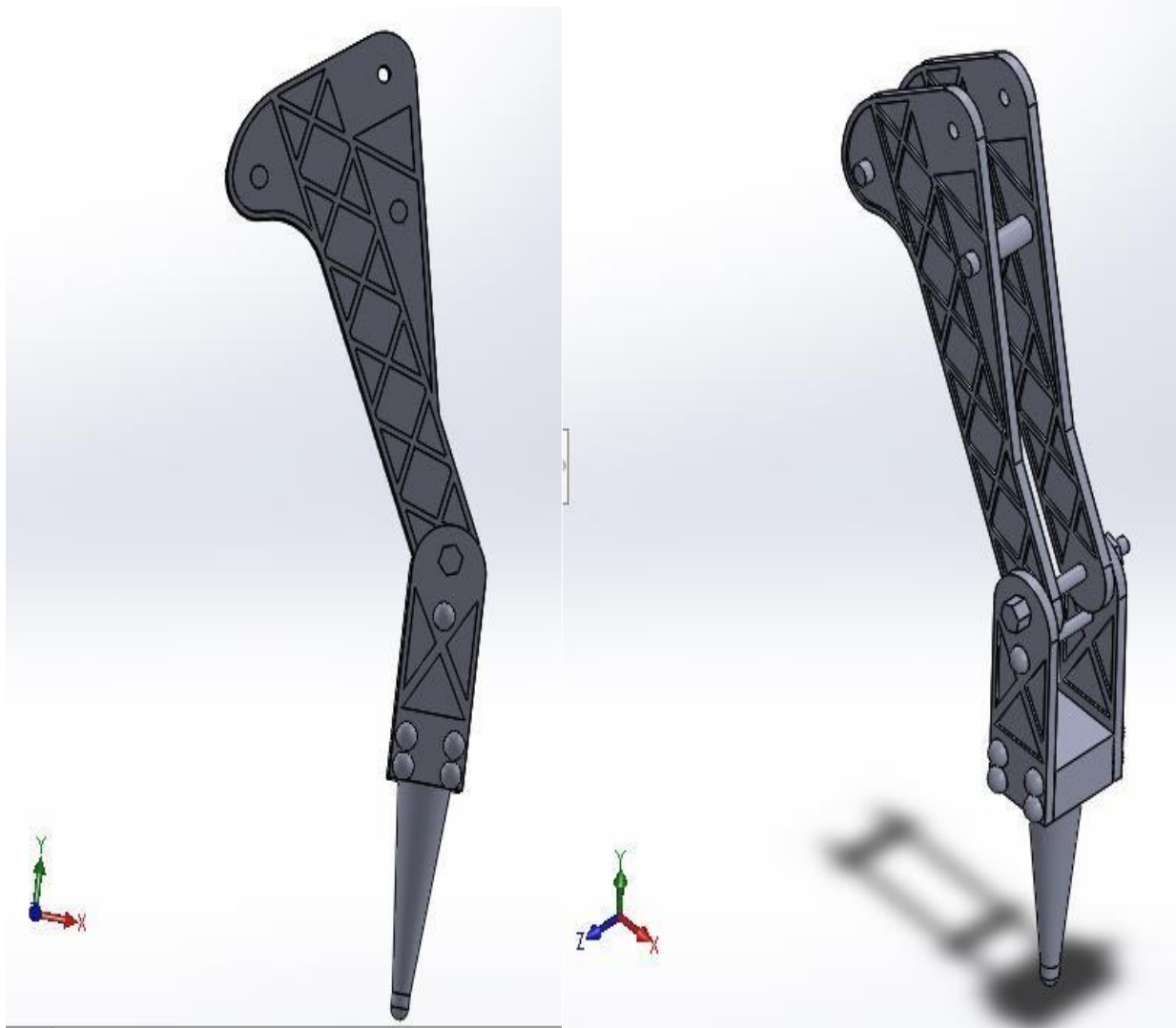
Fig.3. Structural design of a leg of the quadruped robot
