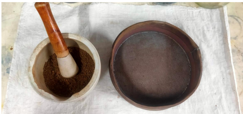
Figure 13: Mortar, pestle and sieve used for soil sample preparation
