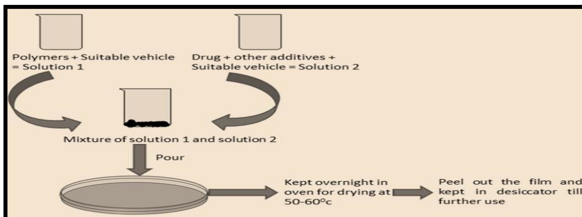
Figure 5.3 Schematic diagram of solution casting method (Source: Kumar and Teotia, 2019)
