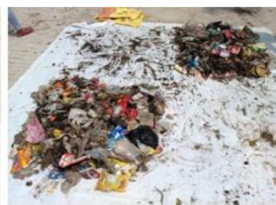
Figure 3: Waste from opposing corners of the divided heap was removed to leave half of the original sample
