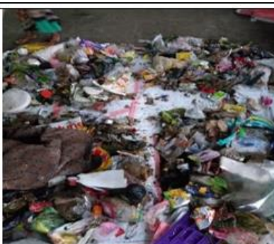
Figure 2: The mixed solid waste is taken; divided into 4 parts, each having 16 kg
