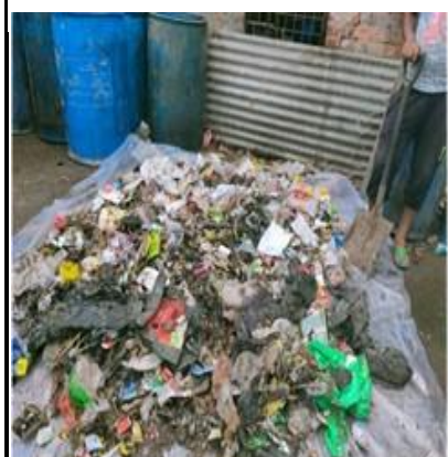
Figure 4: The remaining waste was mixed thoroughly again placed in a clean fresh surface
