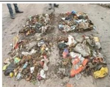
Figure 2: Mixed waste is divided into 4 equal parts each having 16 kg
