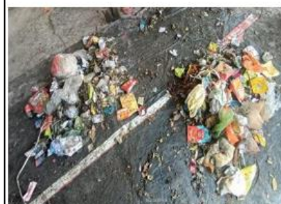
Figure 4: Waste from opposing corners of the divided heap was removed to leave half of the original sample
