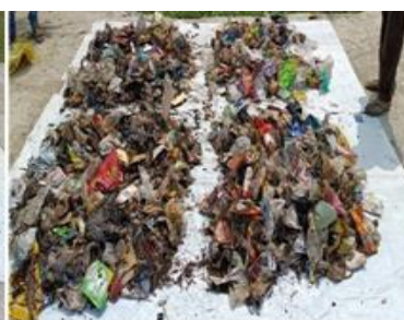
Figure 2: The mixed solid waste taken; divided into 4 parts, each having 16 kg
