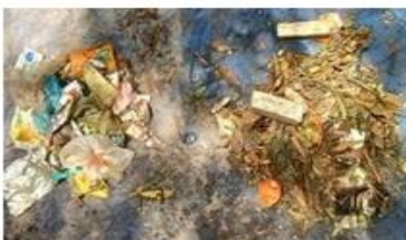
Figure 8: Wastes from opposite corners were mixed & plastic wastes are separated
