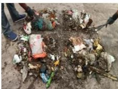
Figure 5: Again, divided into 4 equal parts
