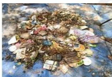
Figure 2: Total 64 kg of mixed solid waste was mixed well for sampling and placed on a clean fresh surface
