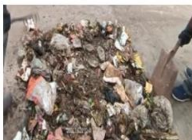
Figure 4: The sample was missed thoroughly again placed on a clean fresh surface in square shape
