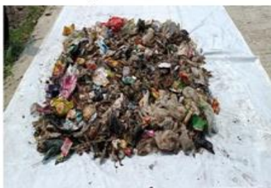
Figure 4: The sample was mixed thoroughly again placed in a clean fresh surface, total weight is 32 kg
