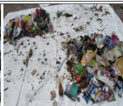
Figure 3: Waste from opposing corners of the divided heap was removed
