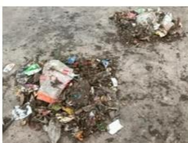
Figure 6: Diagonal portions were taken removing the other 2 portions
