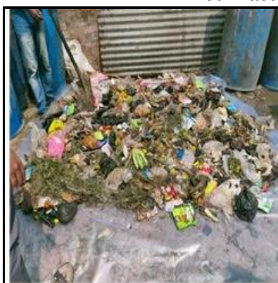
Figure 1: Total 64 kg of mixed solid waste was mixed well for sampling and placed in a clean fresh surface
