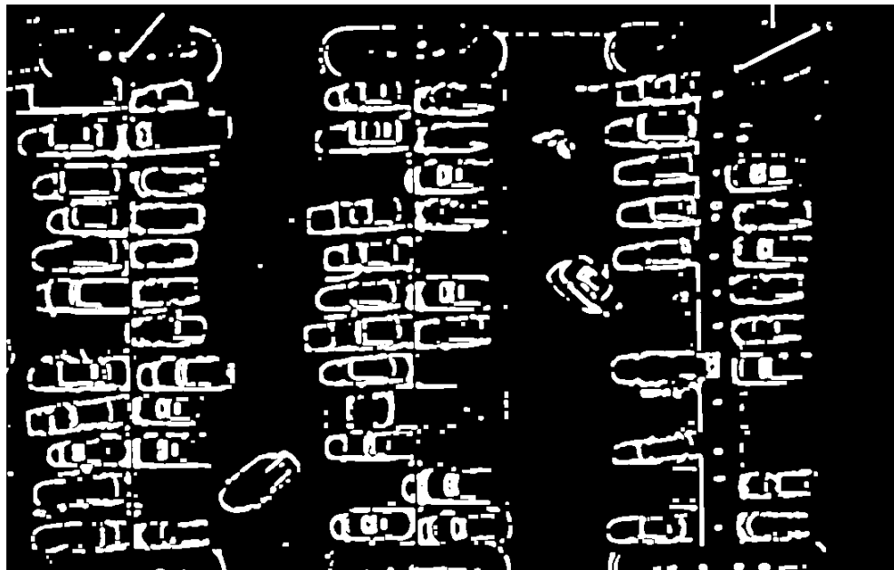
Fig. 16 Median Filtered image undergone dilation in video 1
