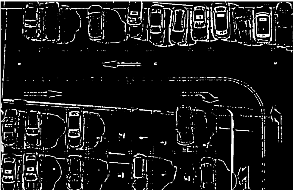
Fig. 14 Resulting image undergoes Median Blur for further noise reduction in video 2
