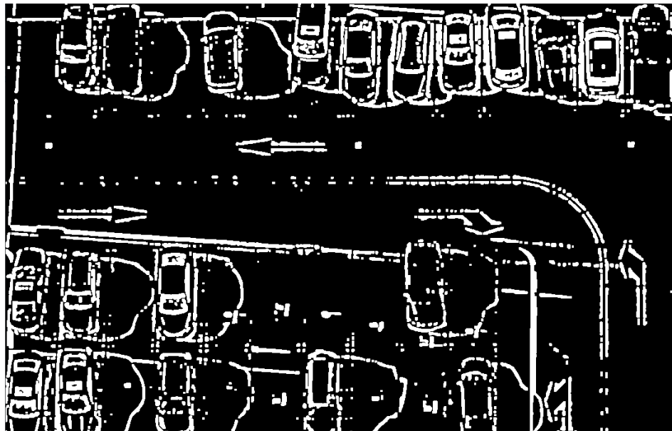
Fig. 17 Median Filtered image undergone dilation in video 2
