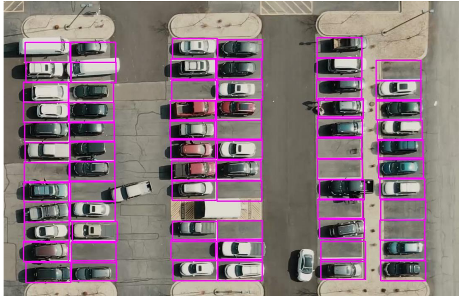
Fig. 1 ROI marked for each parking space in the parking lot in video 1
