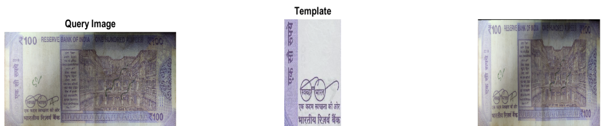
Figure 4.13: Template matching with an unclean Indian 100 Rupee reverse side test image in presence of shadow
